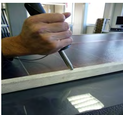
Fig. 7: Accessibility test with artificial finger and cutting test
