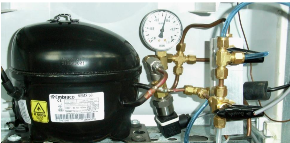
Fig. 6: Variable compressor with filling system
