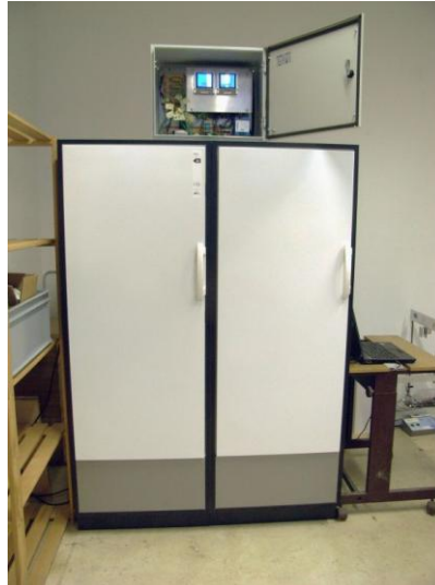
Fig. 8 Original refrigerator (left) and modified refrigerator (right) built into the same cabinet with data acquisition equipment on top
