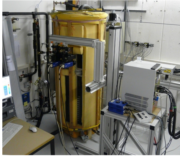
(b) In situ TES with the laser and cameras mounted on the QFV translation system to the right.
