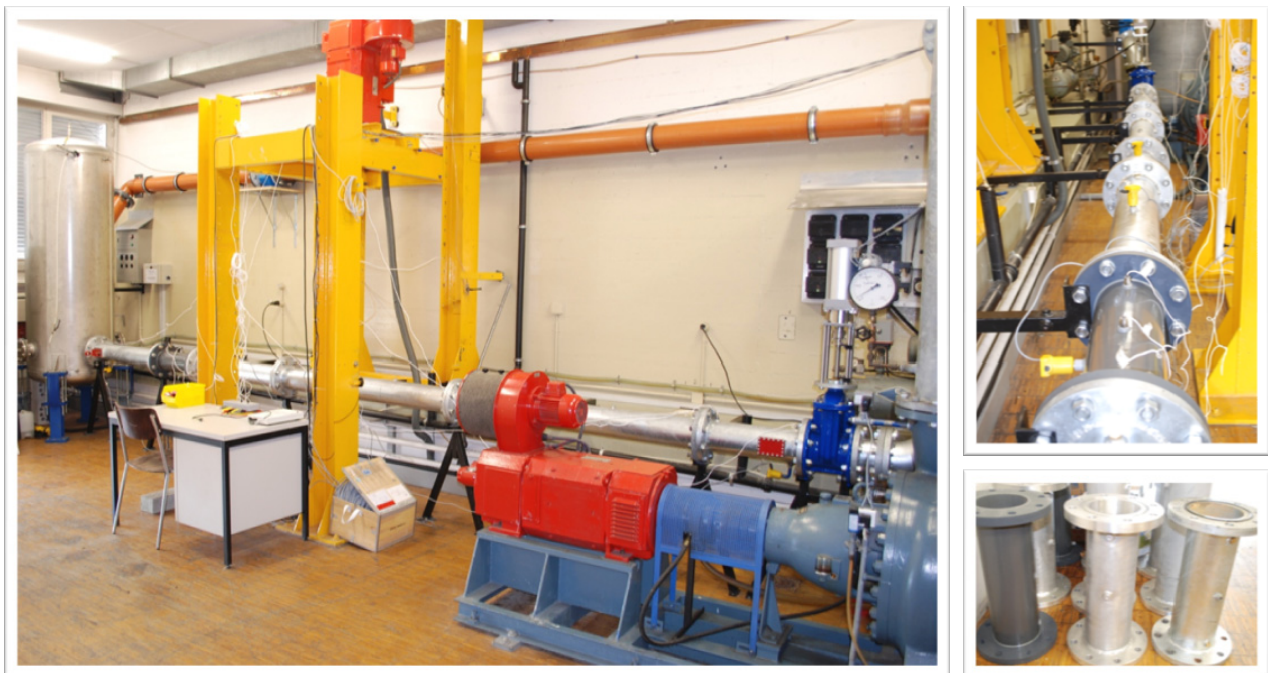
Figure 6.1 : Photos of the physical scaled model with the steel, PVC, and aluminum reaches
