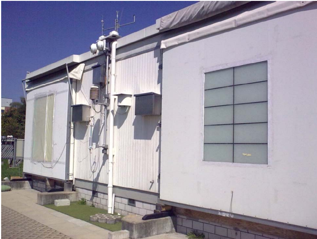
Figure 7: Solar Radiation calorimeter at EMPA.
