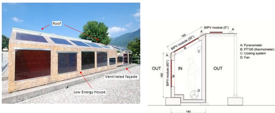
Figure 1: BiPV test stand: external and internal view.
