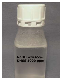
Figure 17: Precipitation in case of DHSS 1000 ppm and NaOH 45 wt.% after one month of exposure at room temperature.
