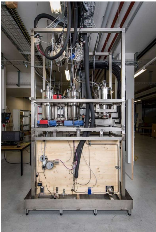
ABSTOREX 1 kW liquid sorption facility
