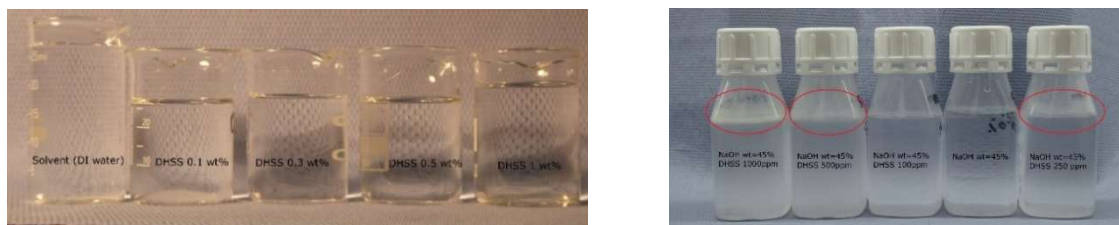
Figure 16: Surfactant (DHSS) solutions with different concentration after preparation (left) and after one week of ageing at room temperature (right) - visible modifications in case of solutions with DHSS concentration higher than 250 ppm.
