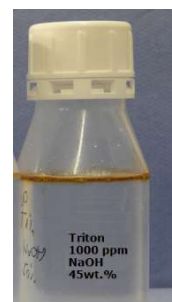
Figure 18: Surfactant phase separation after 48 days at room temperature in case of Triton 1000 ppm and NaOH 45 wt.%.
