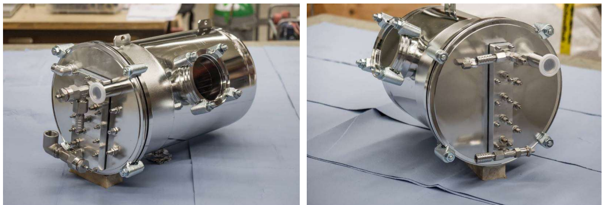
Figure 29: E-C (left) and A-D (right) heat and mass exchanger in its container.
