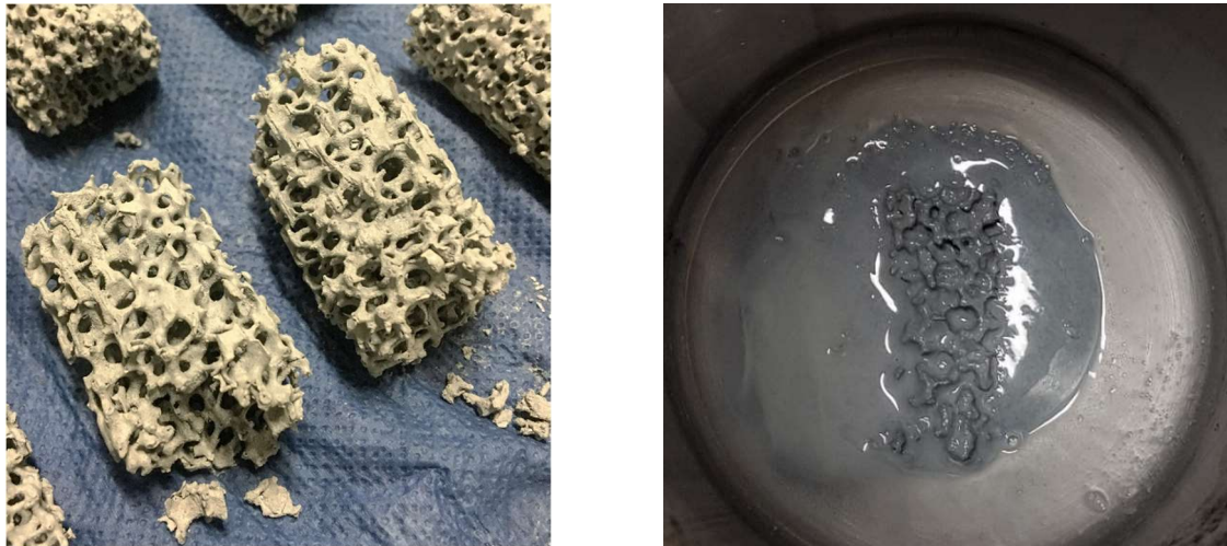
Figure 21: Left: ceramic foam after one month of lye exposure (colour change and crumbling); right: dissolved ceramic foam sample after a two-month immersion in concentrated sodium hydroxide.
