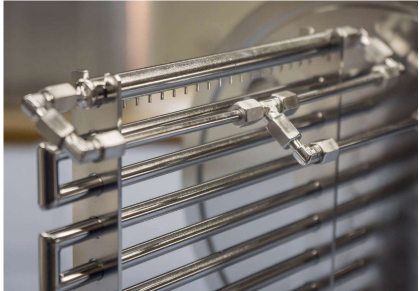
Figure 26: Isometric view of the Absorber-Desorber heat and mass exchanger with dismountable hair-pins (tube bundle and flange in blue, manifold in yellow, left) and associated picture of the built heat and mass exchanger (right).
