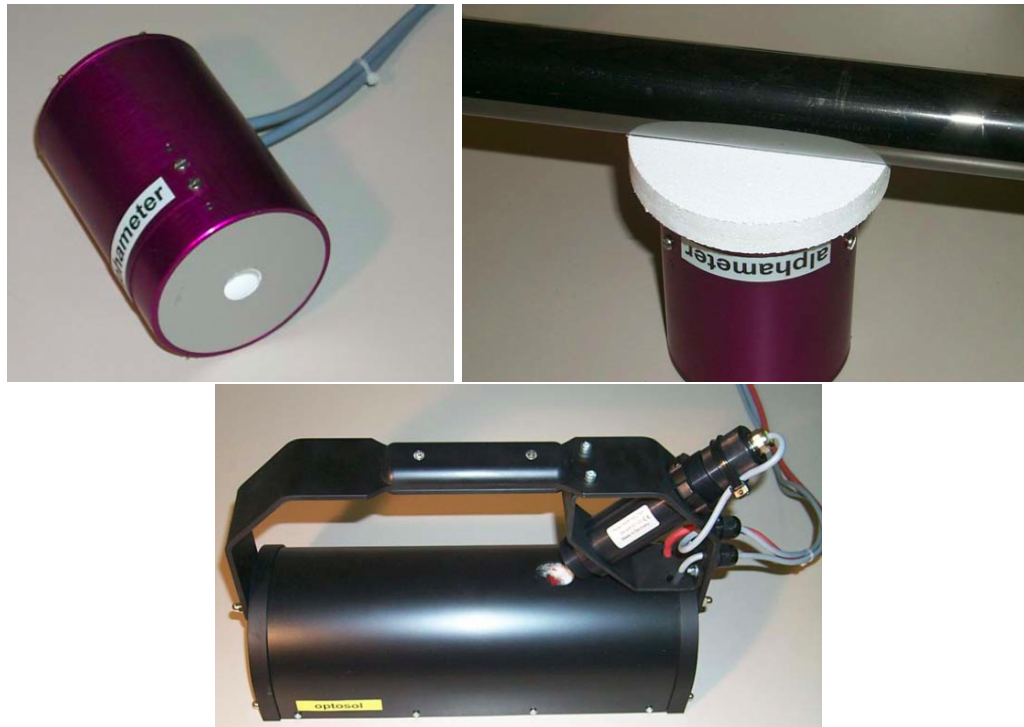
Figure 13: The alphameter (upper two pictures) from Optosol GmbH is a low resolution spectrometer that measures the reflection of selective absorbers in the wavelength range from 0.3 \mu\text{m} to 1.9 \mu\text{m} . The emissiometer (lower picture) measures the reflected thermal radiation at 70^\circ \text{C} [50].
