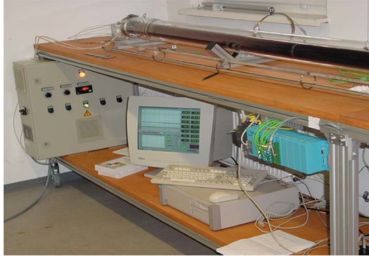
Figure 9: ThermoREC: Thermal loss measurement test bench of DLR, where the absorber tube of the receiver is heated to a desired temperature and the thermal losses are determined [44, 45].
