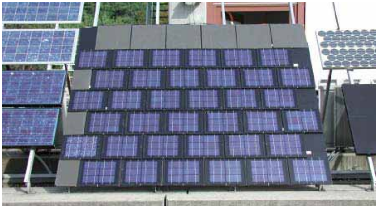
The photo shows the test stand of the latest generation of developed roof shingles Sunplicity at LEEE in Lugano (Photo LEEE).
