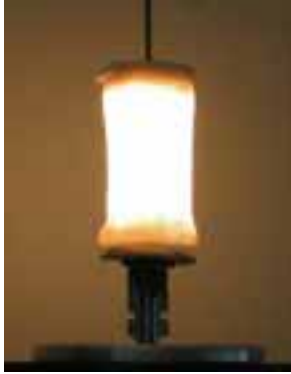
Fig. 2: Incandescent mantle emitter made from \text{Yb}_2\text{O}_3 .
