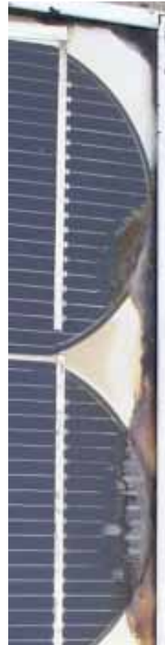
Picture 2: sealant infiltration
