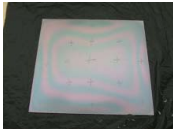
Figure 4: Picture of layer L180602/4 deposited at 135.6 MHz and 10.4 Å/s. Each fringe represents a change in thickness of ca. 600 Å (of an average thickness of roughly 6000 Å).
