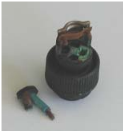
Figure 4: burned cable and damaged connector
