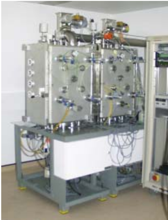
Fig. 1: Single chamber 30x30 cm 2 VHF plasma deposition installation at IMT (DOIT project; photo: IMT / Univ. NE)
