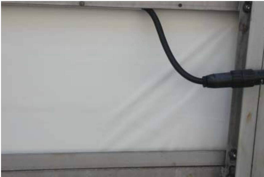
Figure 1: wrinkles caused by Tedlar detachment from aluminium foil.
