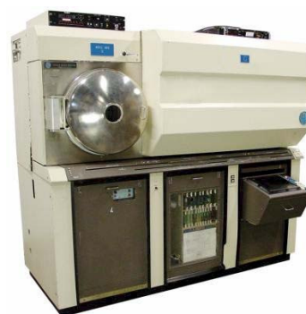
Figure 2: MRC sputterer for the deposition of the front and rear contacts on 30 x 30 cm 2 CIGS thin-film solar cells (photo: ETHZ)
