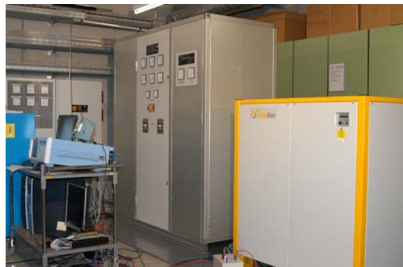
Figure 6: 100 kW solar generator simulator with a 100 kW inverter from Sputnik (photo: BFH-TI).
