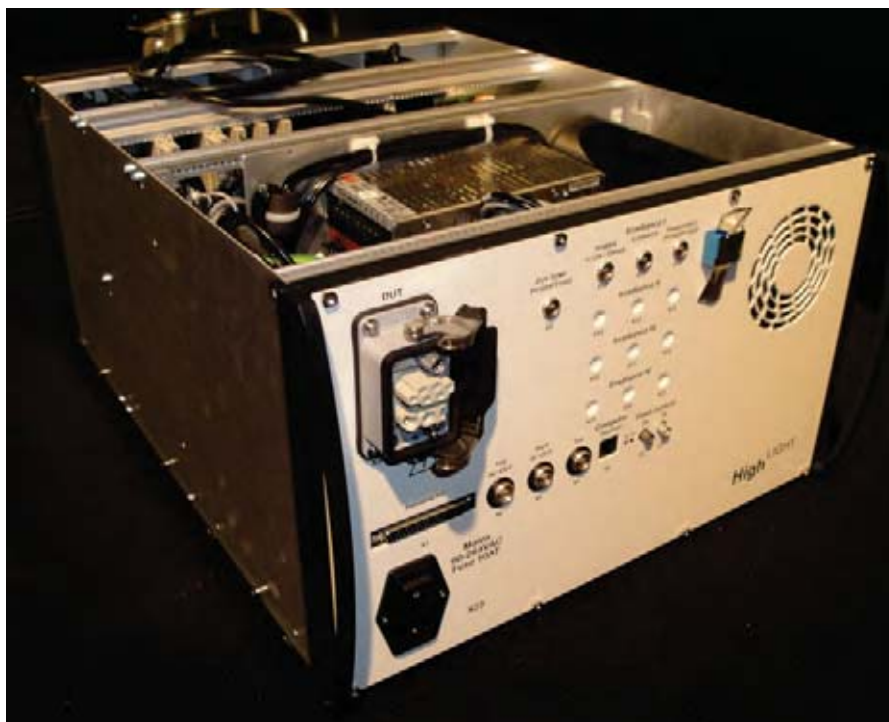
Figure 1: prototype of the novel MPVT electronic load (EL) manufactured by Pasan SA.
