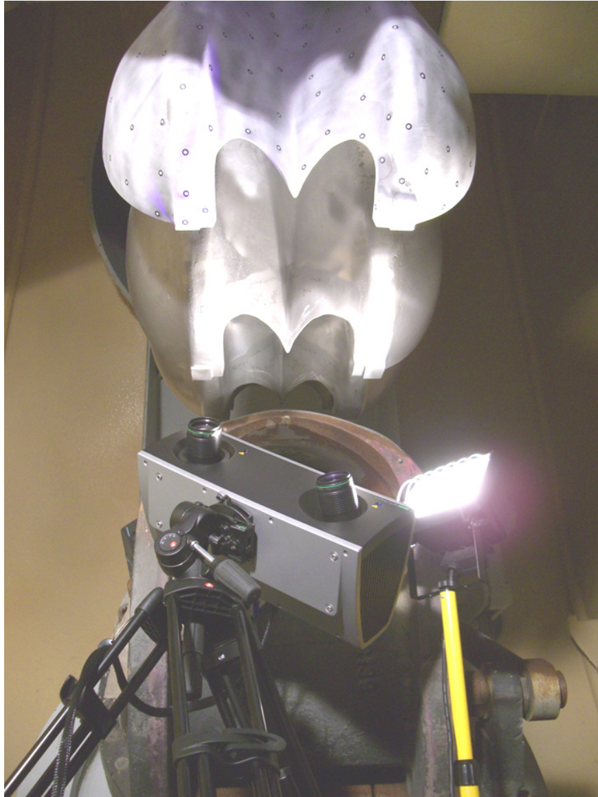
Fig. 7. Digitizing of Pelton buckets geometry in the power plant: Special camera mounted on a tripod below the buckets of the runner with stick-on reference points.
