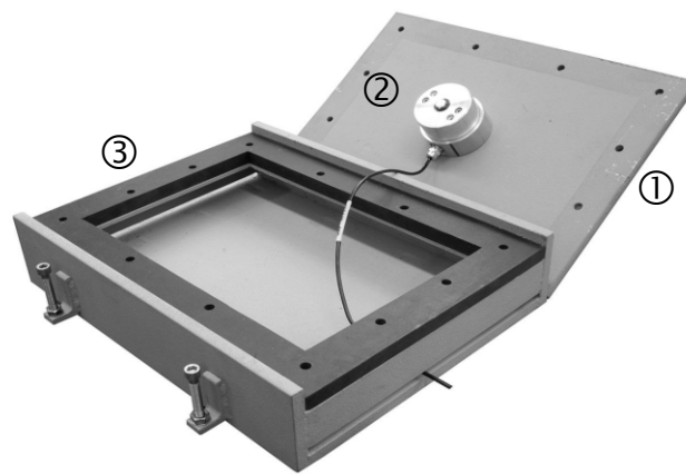
Figure 1: Swiss plate geophone system with steel plate ① (before assembly), geophone sensor ② and elastomer bearing ③ on the aluminum casing (VAW)
