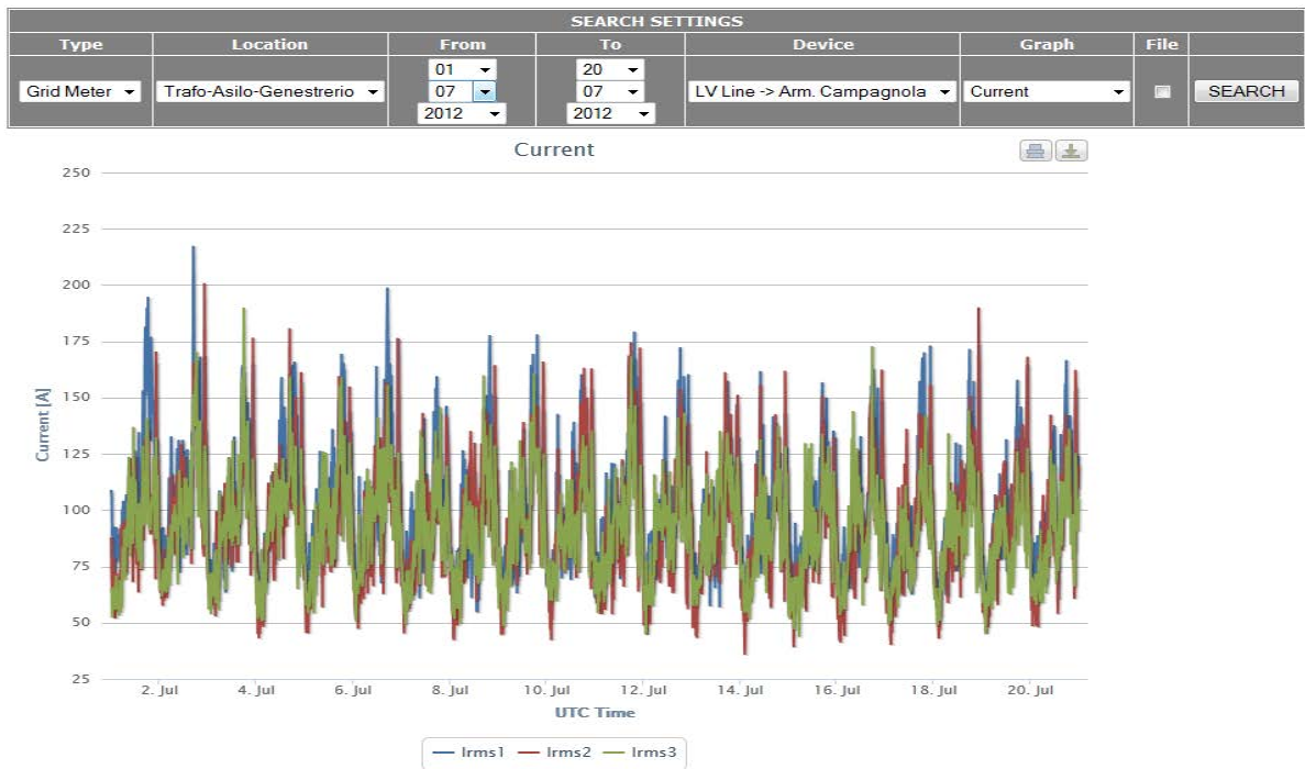
Figure 79: Example of current measurements at a transformer branch
