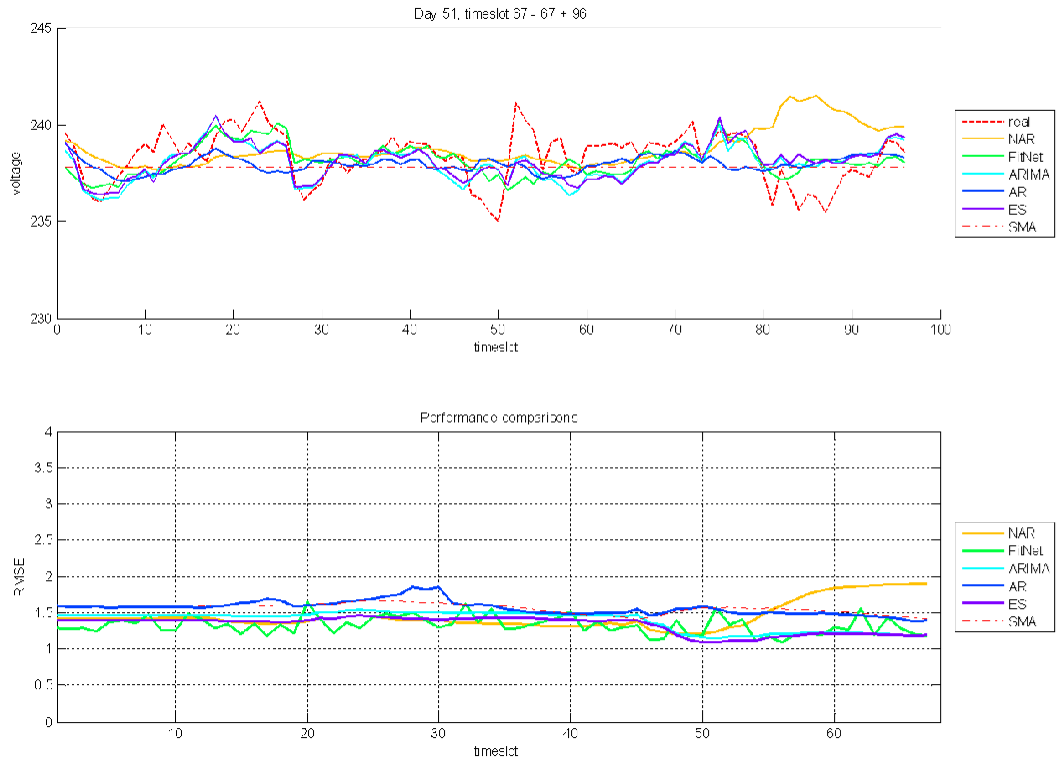
Figure 44: Qualitative and quantitative comparisons. The above image is the real voltage (in red dotted line) versus the forecast ones. The below figure is the change of rootmean-square-errors of these methods.
