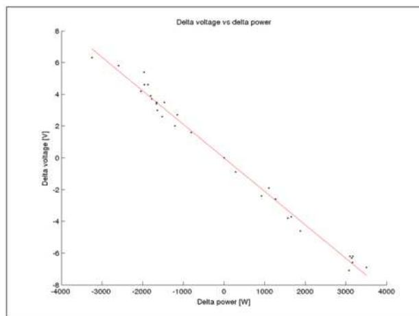
**Figure 29: voltage drops depending on differences in absorbed power. Voltage drops exhibit a quite neat linear relationship of about 2 Volts per kW.**
