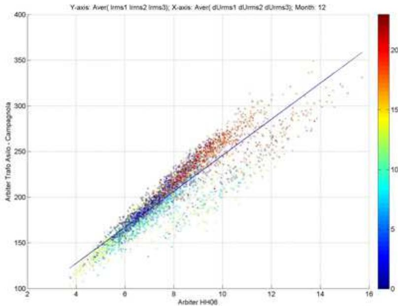
**Figure 25: Phase currents at the Asilo transformer with direction towards HH06 (y-axis) and the phase voltage difference between HH06 and the Asilo transformer voltages (x-axis) (all three phases shown) in 10-minute intervals of all measured days of the month of December. The colors indicate the (UTC) time of day when the point was measured.**
