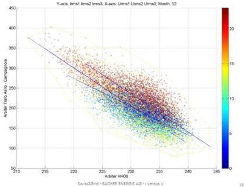
**Figure 23: Phase currents at the Asilo transformer with direction towards HH06 (y-axis) and the phase voltage at the HH06 (x-axis) (all three phases shown) in 10-minute intervals of all measured days of the month of December. The colors indicate the (UTC) time of day when the point was measured.**
