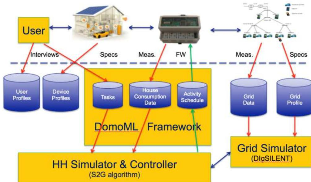
Figure 11: the DomoML framework interfacing User, Algorithm, and HAC within the system architecture
