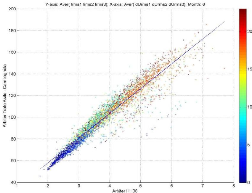
**Figure 24: Phase currents at the Asilo transformer with direction towards HH06 (y-axis) and the phase voltage difference between HH06 and the Asilo transformer voltages (x-axis) (all three phases shown) in 10-minute intervals of all measured days**
