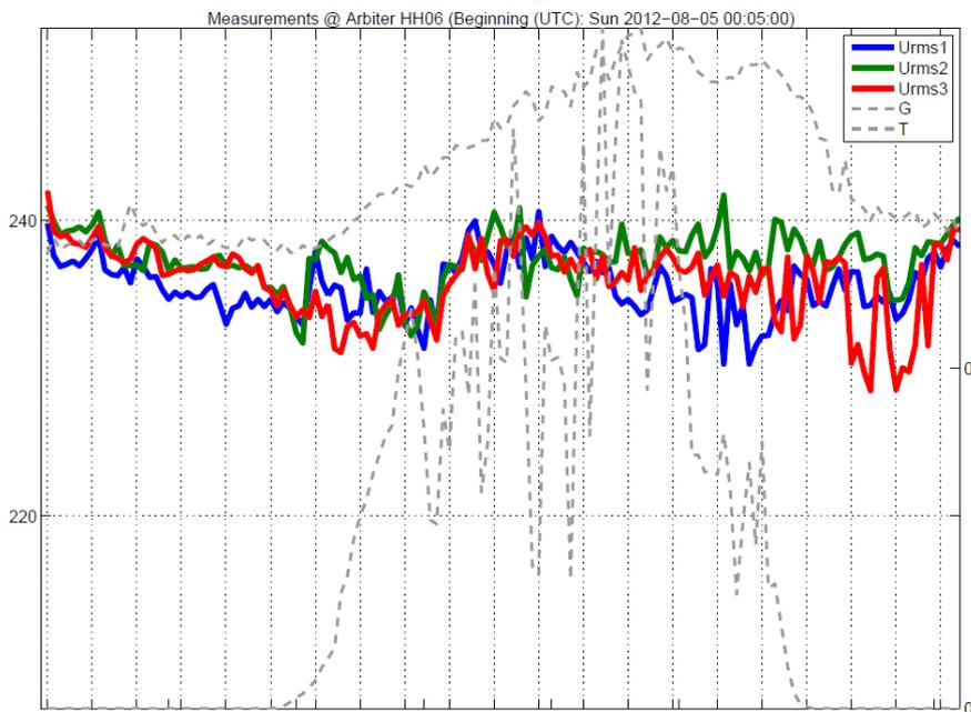
Figure 20: x-Axis: Example of measurements at HH06 in 10-minute intervals of a single day (Sun 2012-08-05, beginning at midnight); y-axis (left side: voltage magnitudes [V] of the three phases (red, blue, green); right side: Temperature (normalized T, upper dashed line) and sun shine (normalized G, lower dashed line)
