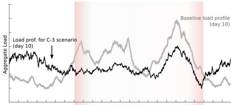
**Figure 28: detailed results for the Baseline and C-3 case. The overall network load at the MV-LV transformer is reported for day 10. The overall load is substantially flattened with a remarkable load shift towards periods with low price of energy.**
