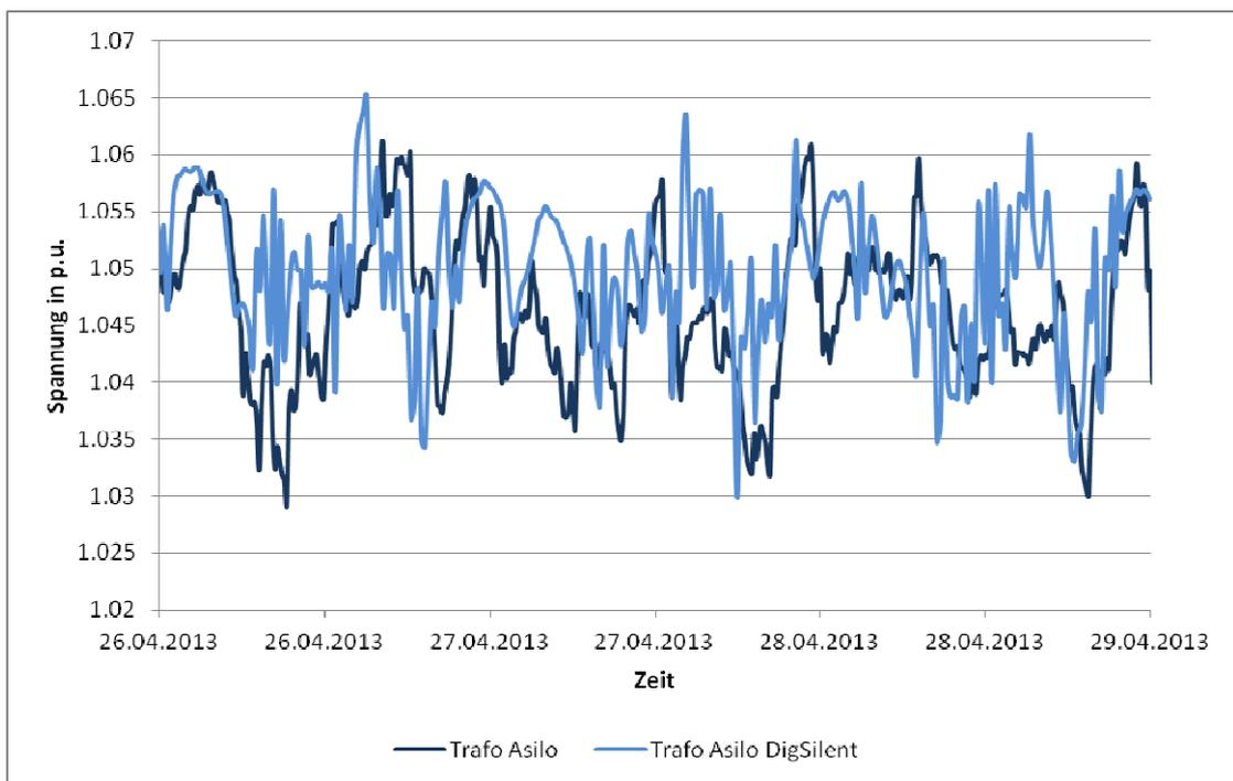
**Figure 37: comparison of voltage between simulated and measured string**
