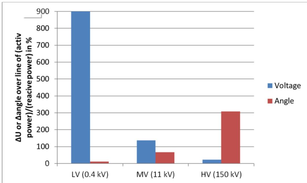
**Figure 34: effect of power in different grid levels**
