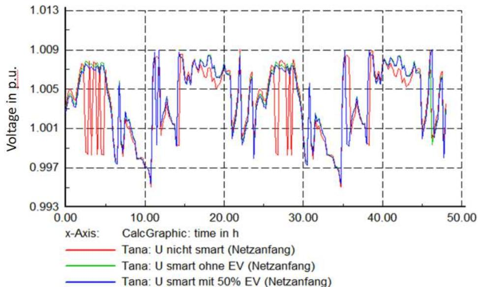
**Figure 46: run of the voltage [p.u.] at the MV/LV transformer in Mendrisio when implementing smart households with and without EV with automatic transformer taps**
