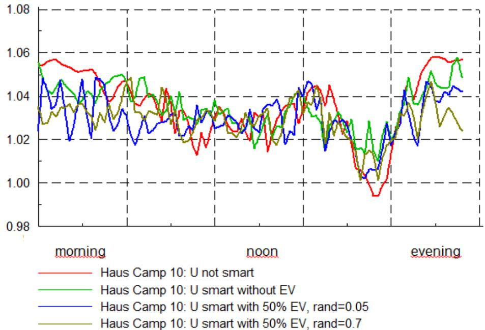
**Figure 43: run of the voltage [p.u.] at end of a low voltage string in Meiringen with maximal penetration of smart HH and by varying EV use and randomisation factor**
