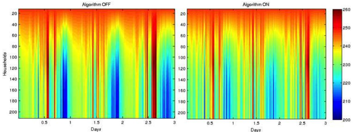
**Figure 30: 220-households simulation: representation of voltages (colors: blue: low, red: high) according to the position of the household along the distribution network (y axis) and time (x axis). Left plot shows behavior when the algorithm is switched off, compared with the behavior when the algorithm is on (right plot). Note that the algorithm reduces extreme voltages.**
