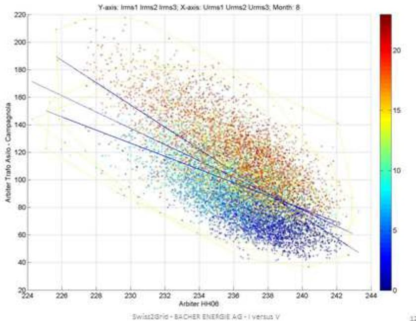
**Figure 22: Phase currents at the Asilo transformer with direction towards HH06 (y-axis) and the phase voltage at the HH06 (x-axis) (all three phases shown) in 10-minute intervals of all measured days of the month of August. The colors indicate the (UTC) time of day when the point was measured.**
