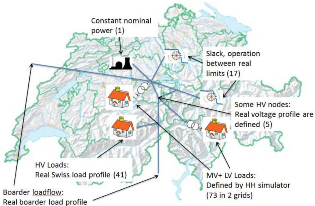
**Figure 39: Loads and production in the different grid levels**
