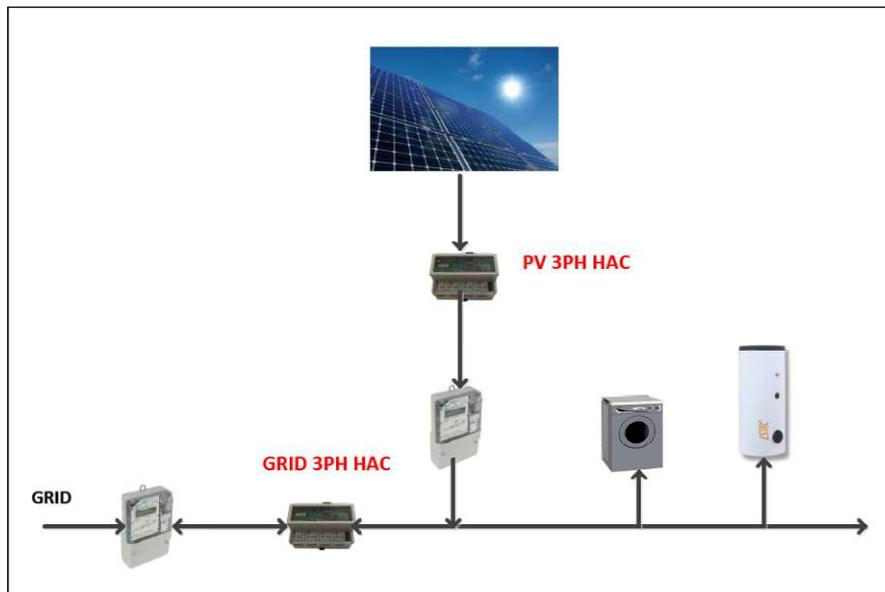
**Figure 3: connection of PV HAC and Main HAC**
