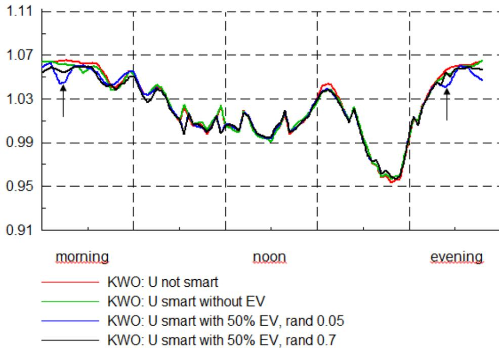
**Figure 41: run of the voltage [p.u.] at the end of a low voltage sting when implementing only one smart load (equal to 5 HH) and by varying EV use and randomisation factor at the end of the string**
