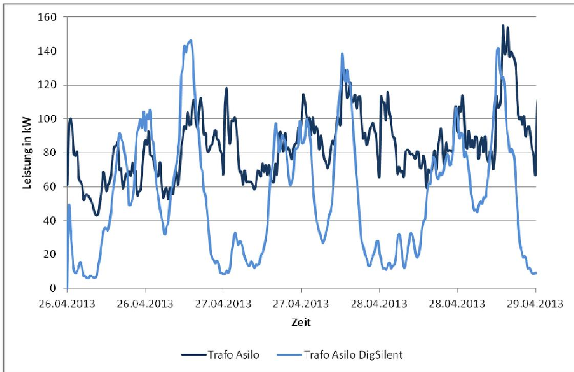
**Figure 36: comparison of power between simulated and measured string**
