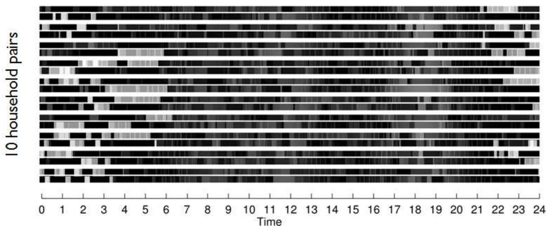
**Figure 27: a detailed representation of a C-2 scenario. Pair of households are enabled to communicate among them. Bright timeslots represent moments in which a high power is drawn from the network.**
