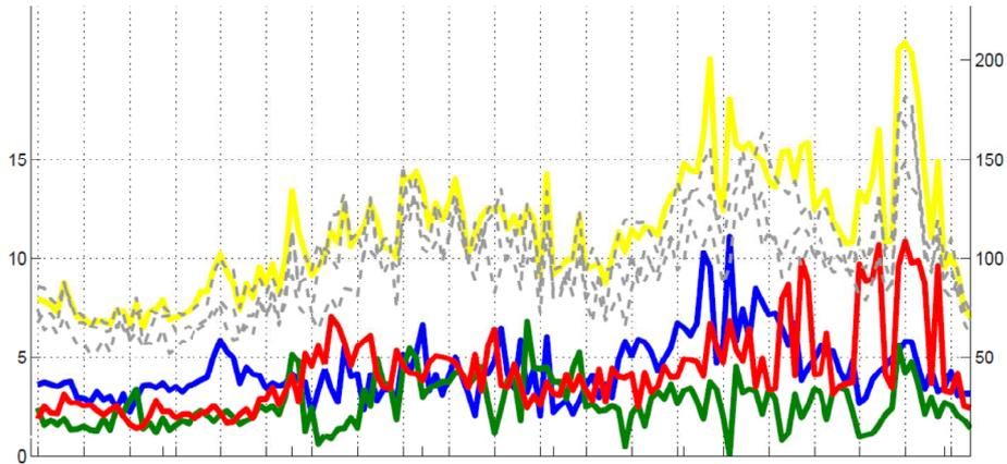
**Figure 21: x-Axis: Example of (left side y-axis) voltage phase differences of HH06 plug to Asilo transformer plug in 10-minute values of a single day (Sun 2012-08-05, beginning at midnight) and the (right side y-axis) currents at the transformer low voltage side. y-axis (left side: voltage differences of the three phases (red, blue, green); right side: currents measured at transformer).**
