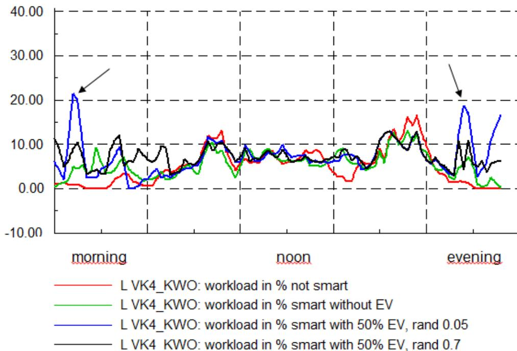
**Figure 42: run of the active power [kW] on a low voltage line when implementing only one smart load (equal to 5 HH) and by varying EV use and randomisation factor at the end of the string**
