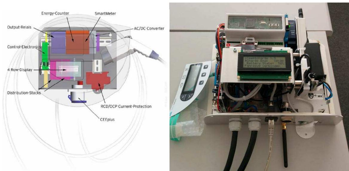
**Figure 9: EV Home Charge Device (HCD) with an HAC**
