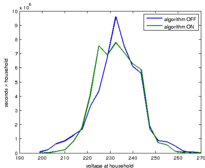
**Figure 31: the plot reports the amount of time (y axis) that a given voltage (x axis) was measured during the simulation reported in Figure 11. Blue plot reports results when algorithms were turned off, whereas green plot reports results with active algorithms.**
