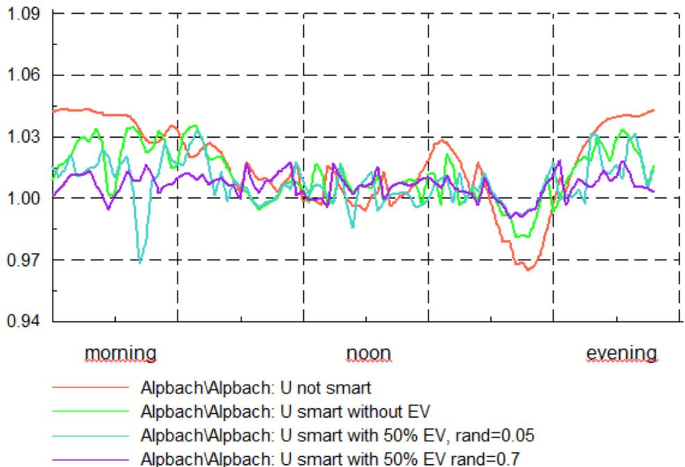
**Figure 44: run of the voltage [p.u.] at a medium voltage busbar in Meiringen with maximal penetration of smart HH and by varying EV use and randomisation factor**
