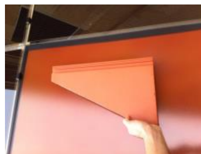
• Figure 5 : addition of a colored encapsulant at the back of semi-transparent a-Si cell enables device color tuning
