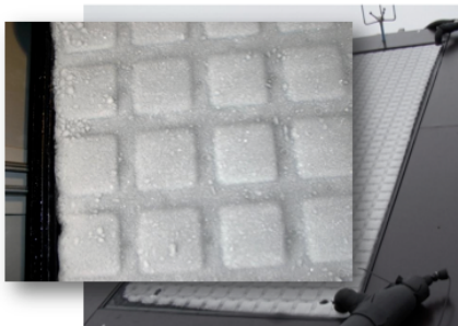
Fig. 8: frost on a selective uncovered collector when used below the dew point (source SPF, 2011)
