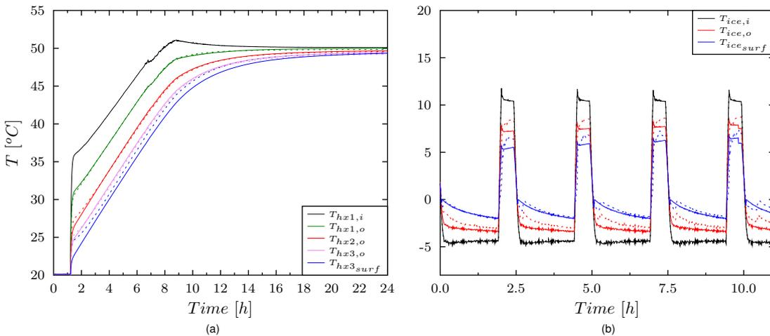
Figure 4: Immersed heat exchanger temperatures for a) forced heating (FH) and b) ice and de-ice (IDI). Solid lines are used for numerical calculations and dashed lines for experimental data.
