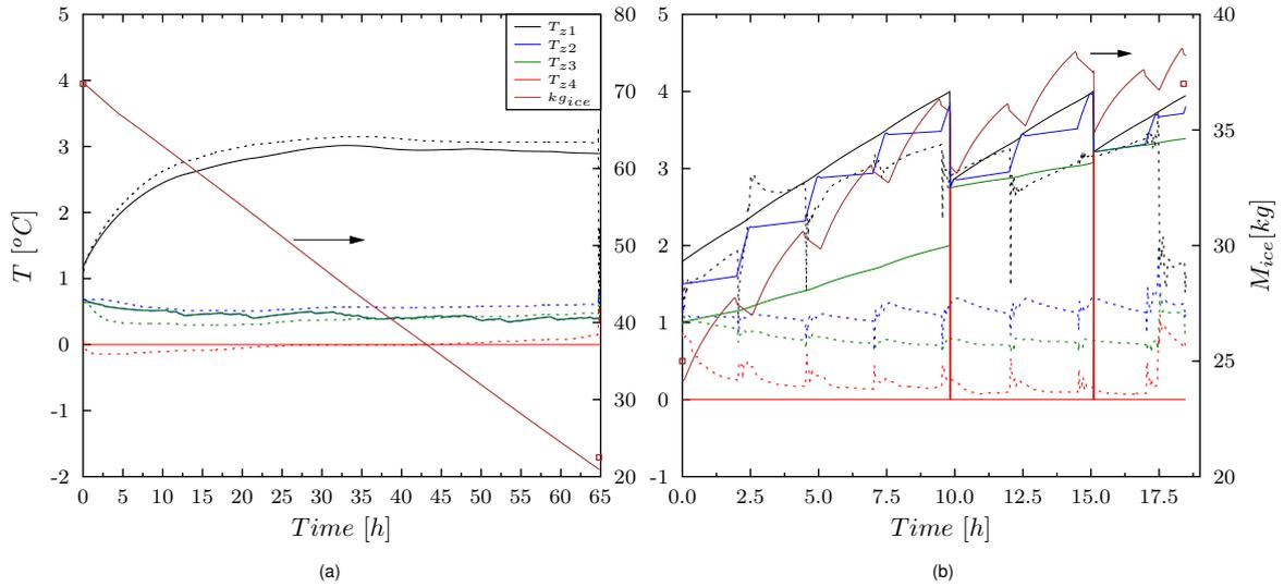
Figure 3: Storage tank temperature (left axes) and mass of ice in the store (right axes) for a) natural melting (NM) and b) ice and de-ice (IDI). Solid lines are used for numerical calculations and dashed lines and symbols for experimental data.
