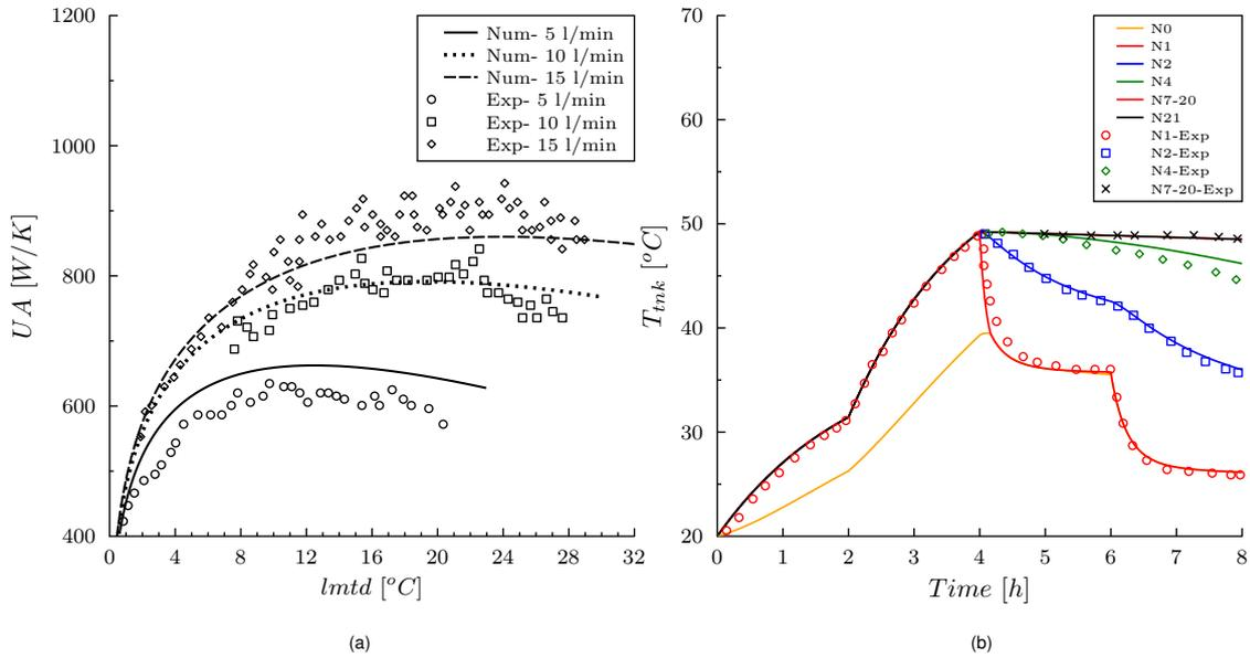
Figure 1: a)  $UA$  of the heat exchanger compared to experiments from [2] and b) storage tank temperatures compared to experiments from [3]. ( $lmtd$  = logarithmic mean temperature difference)
