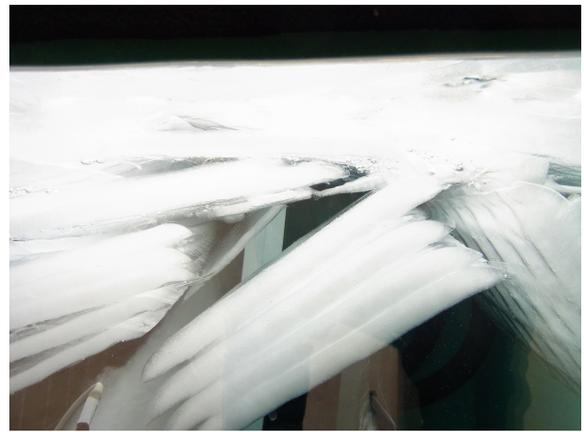
Figure 2: Side views into the ice storage in the SPF lab a) wall heat exchangers (left) and heat exchanger that can be de-iced (right) and b) accumulated ice layers at the storage's water surface after several icing and de-icing cycles (thickness of layers  $\sim 2$  cm).
