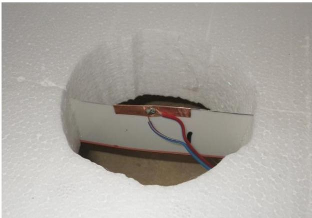
Figure 7. T-type fine-wire thermocouples soft-soldered to self-adhesive copper foil tape strips fixed to polyester ('Mylar') sheet strips which were mounted vertically in the calorimeter's air ports.
