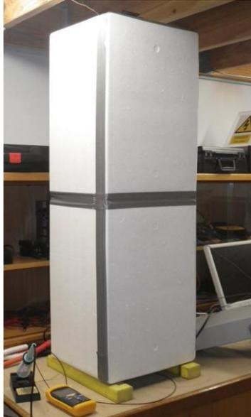
Figure 5. Overall appearance of the experimental two-chamber calorimeter, with controlled temperature laboratory air drawn through a circular aperture in the bottom chamber via a similar aperture in the top chamber, using a speed-controlled centrifugal blower.
