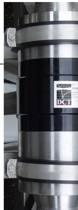
Pressure Amplifier: Source inlet connected to supply (centre left), main entry (bottom) and exit (top) connected to the pressure circuit.
