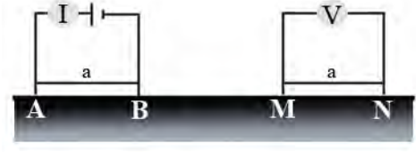
Figure 17: Dipole-Dipole configuration. A and B are the current electrodes while M and N are potential electrodes. \rho_a = \pi n(n+1)(n+2)aR . Sketch based on [Lowrie, 2007].
