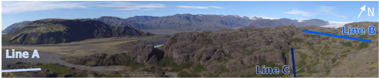
Figure 10: The three geophysical profile lines at Geitafell superimposed on a photograph of the area. All lines start in the host rock (basalt) and end towards the center of the picture in the gabbro.
