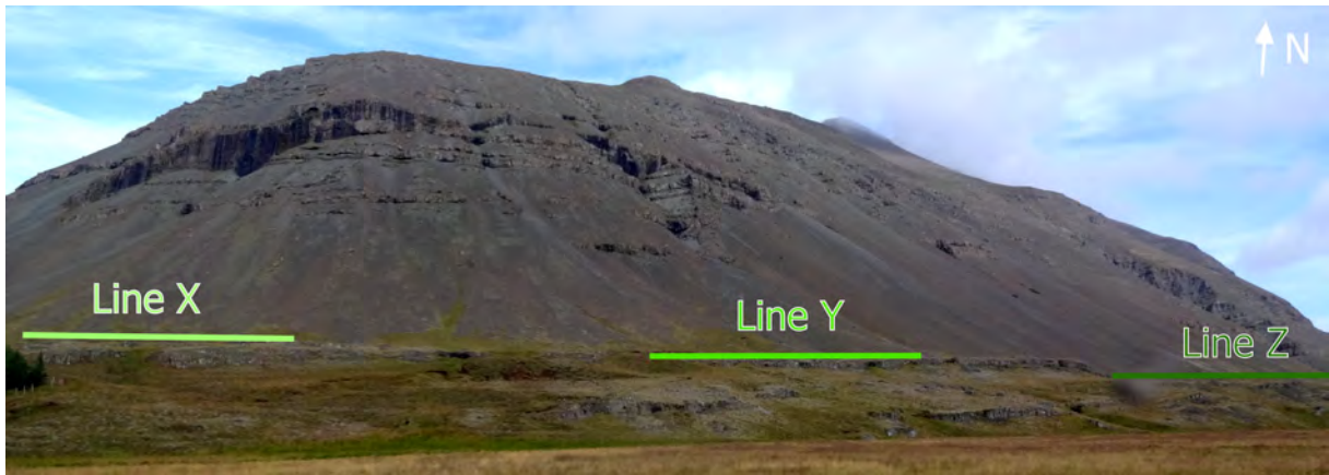
Figure 14: Locations of the three geophysical profile lines at Hoffell superimposed on a photograph of the area. Line X is in the actinolite zone; Line Y is in the garnet zone; Line Z is in the epidote zone. The lines in the picture are only drawn approximately on their real locations.
