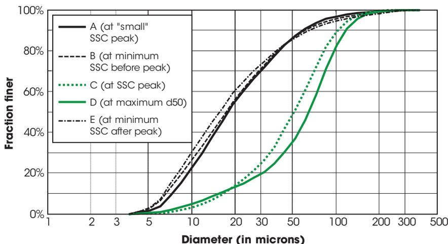
Selected particle size distributions measured in the turbine water at times indicated in Figure 1 show that particle size varied significantly over time.
