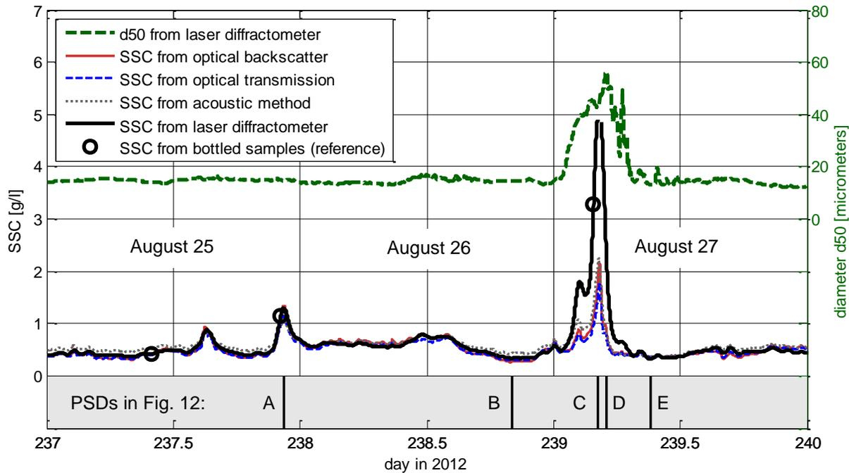
Fig. 11: Time series of SSC in the turbine water, from devices as in Figure 10, reference SSCs from bottled samples, and time series of  $d_{50}$  obtained from LISST; example of three summer days (August 25 to 27, 2012).
