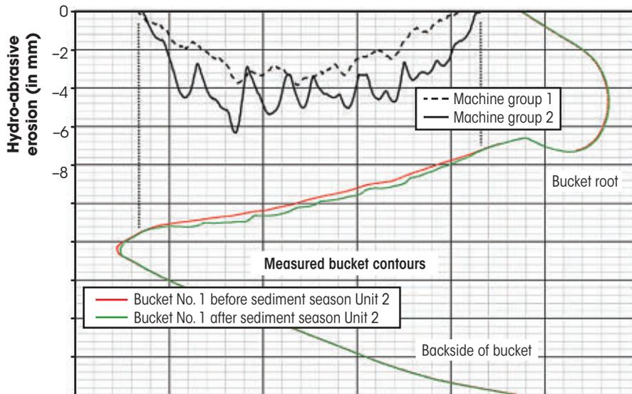
Comparison (black) between the splitter geometries of Bucket 1 of Units 1 and 2 before (red) and after (green) the sediment season reveal a reduction in splitter height on both units.
