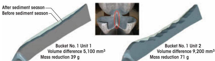
This three-dimensional comparison between the splitter geometries before (transparent) and after (gray) the sediment season for Bucket 1 of Units 1 and 2 shows the change in volume and mass.
