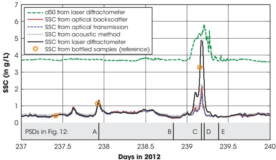
This time series of suspended sediment concentration in the water running through the turbines at the Fieschertal plant provides an example of suspended sediment transport during three summer days in 2012.
