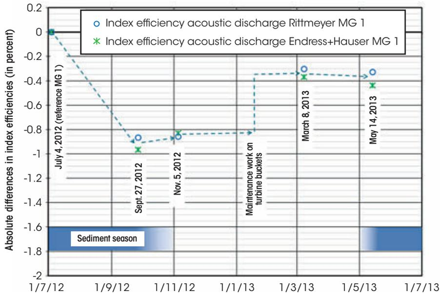
The index efficiency decreased due to hydro-abrasive erosion and increased due to turbine maintenance. Index efficiencies were calculated twice, based on the two available discharge measurements.
