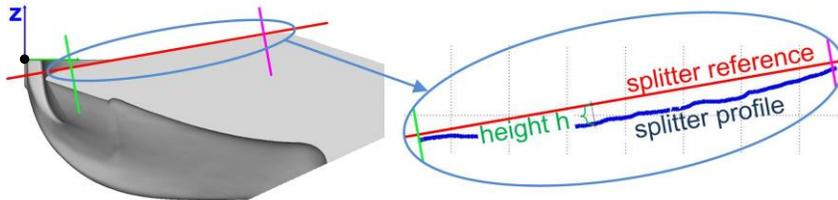
Fig. 3: Definition of eroded splitter height of a Pelton bucket.
