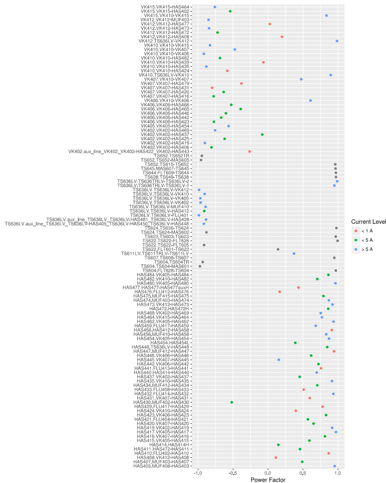
Fig. 7: Power Factor calculation based on measurement data, grouped by current level; data taken on 18.01.2016
