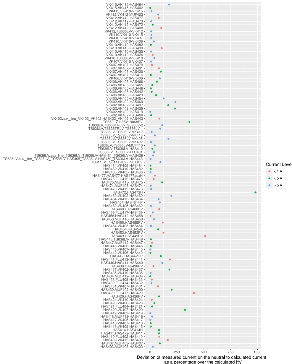
Fig. 8: Neutral current calculation based on phase currents, groups by current level; data taken on 18.01.2016
