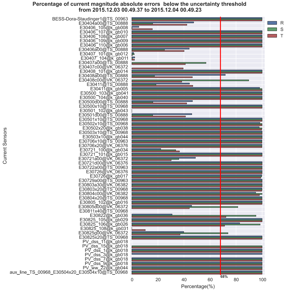
Figure 3: Current Magnitudes: Percentage of absolute residuals between state estimation and measurement of current magnitudes that is below the aggregated uncertainty of measurement and state estimation over a daily time window for 03.12.2015 for each phase of all the compared nodes
