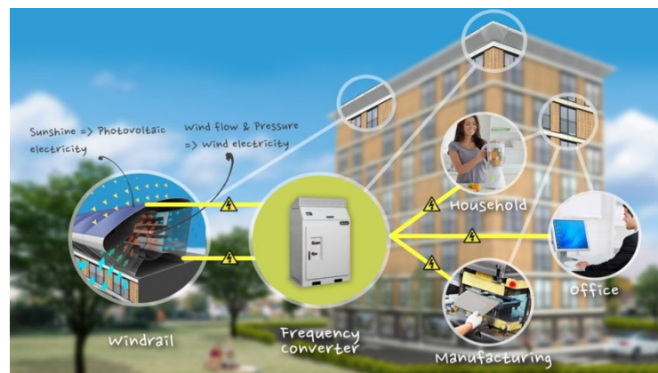
Figure 1: WindRail functional principle
