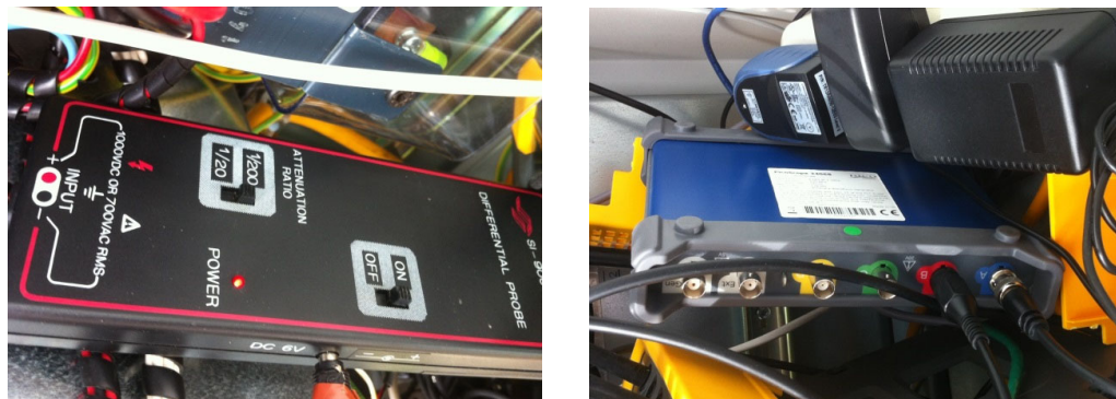
Figure A 2-8: Differential probe configuration and picoscope
