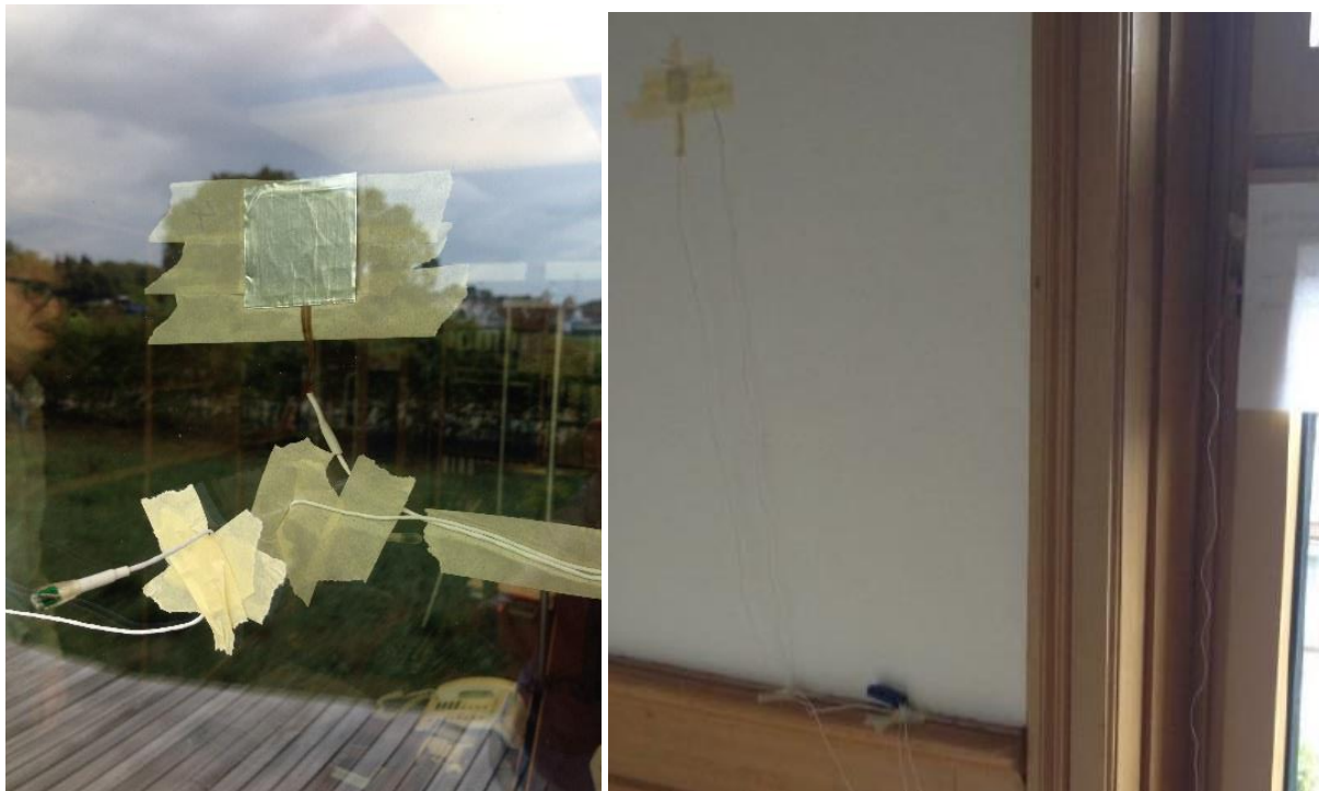
Figure 6: Measurement setup of a window measurement (left) and a wall measurement (right)
