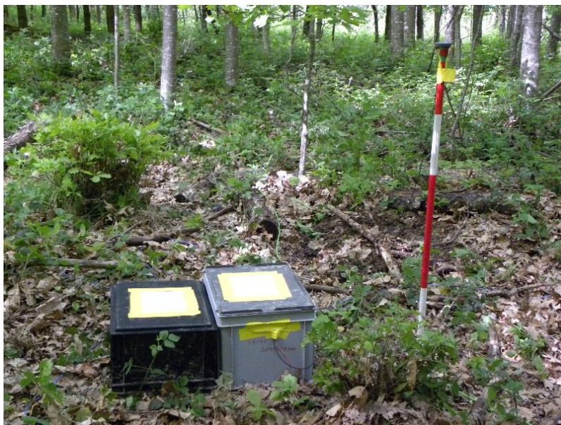
Figure 35 : Magnetotelluric station on the site 3b, in the municipality of Grandcour in spring 2015.
