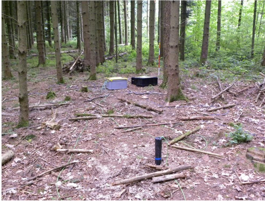
Figure 34 : Magnetotelluric station on the site 3a, in the municipality of Grandcour in spring 2015.
