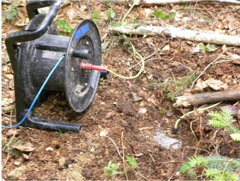
Figure 36 : Example of electrical Ag/AgCl electrode to record the variation of the electrical field over time. Only the grey cap of the electrode is visible on the surface of the ground (right side), while the reel of the 50m cable connects the electrode to the logger (left).
