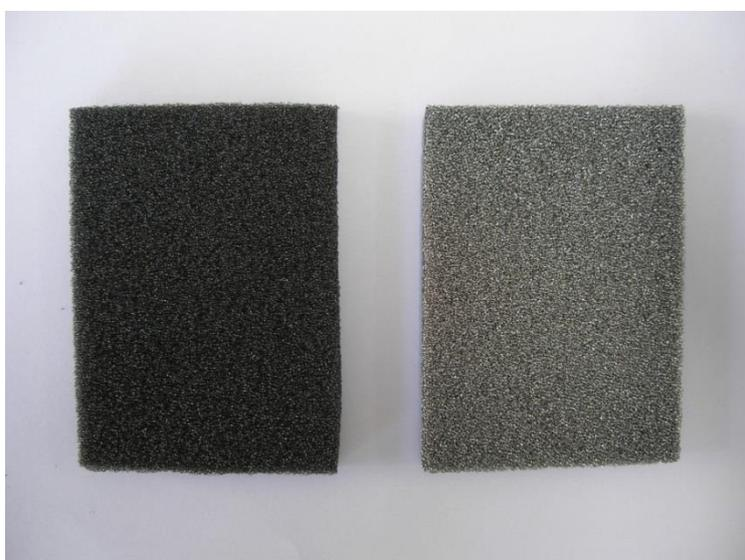
Photo 2: Reticulated vitreous carbon before (on the left) and after sputtering (on the right).
