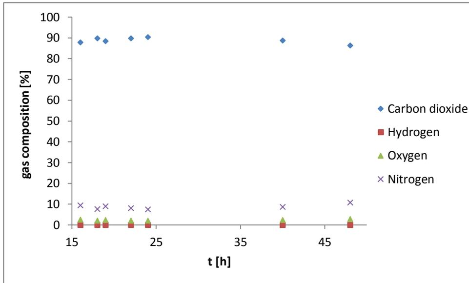
Figure 23: Gas composition in the reactor headspace during the microbial electrolysis cell operation without membrane under 1.3 V of applied voltage.
