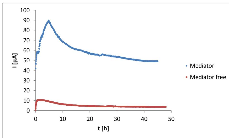
Figure 15: Current monitored using medium containing a mediator and mediator free medium. The anode compartment was not inoculated by *S. cerevisiae* or any other microorganism. The anodic and cathodic compartments were separated by a proton exchange membrane.
