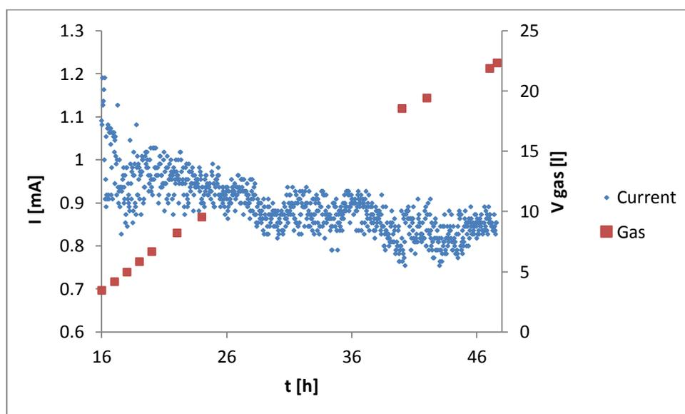
Figure 22: Current and biogas production for the microbial electrolysis cell operated without membrane with 1.3 V of applied voltage.
