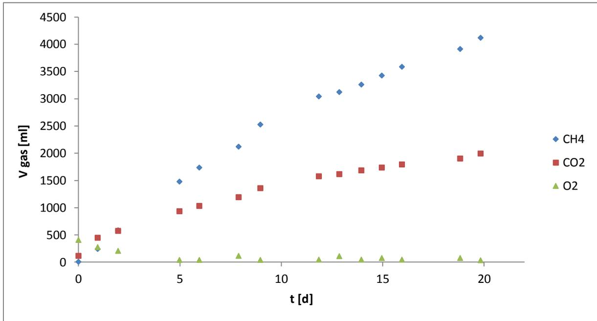
Figure 63: Gas production over the acclimation phase preceding the digestion of fermentation waste under 1.5V.
