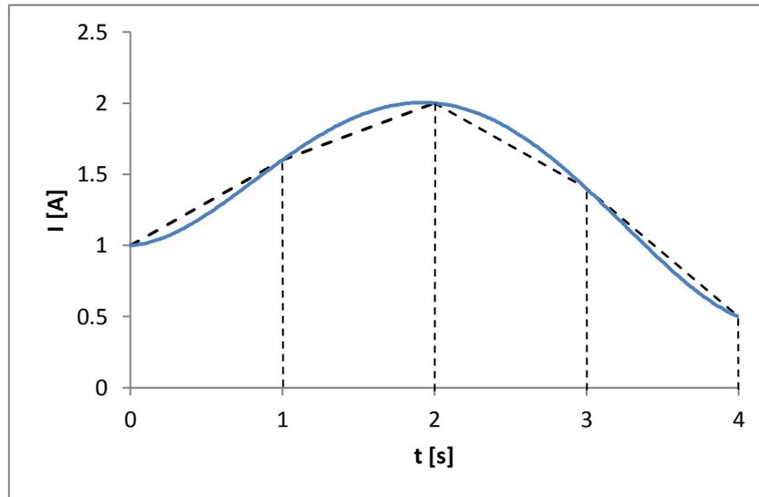
Figure 10: Representation of the trapezoidal rule integration method. The region under the curve was segmented into multiple trapezoids.
