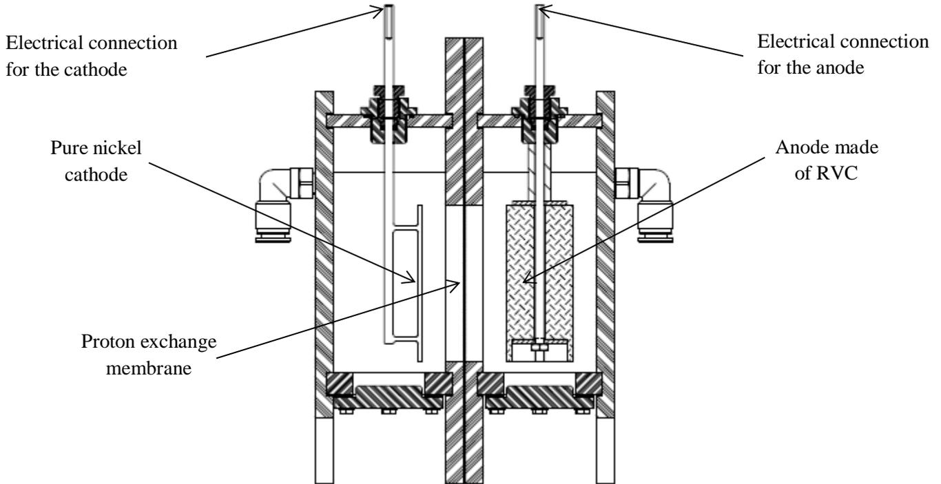
Figure 5: Set up of the fuel cell with anodic and cathodic compartments
