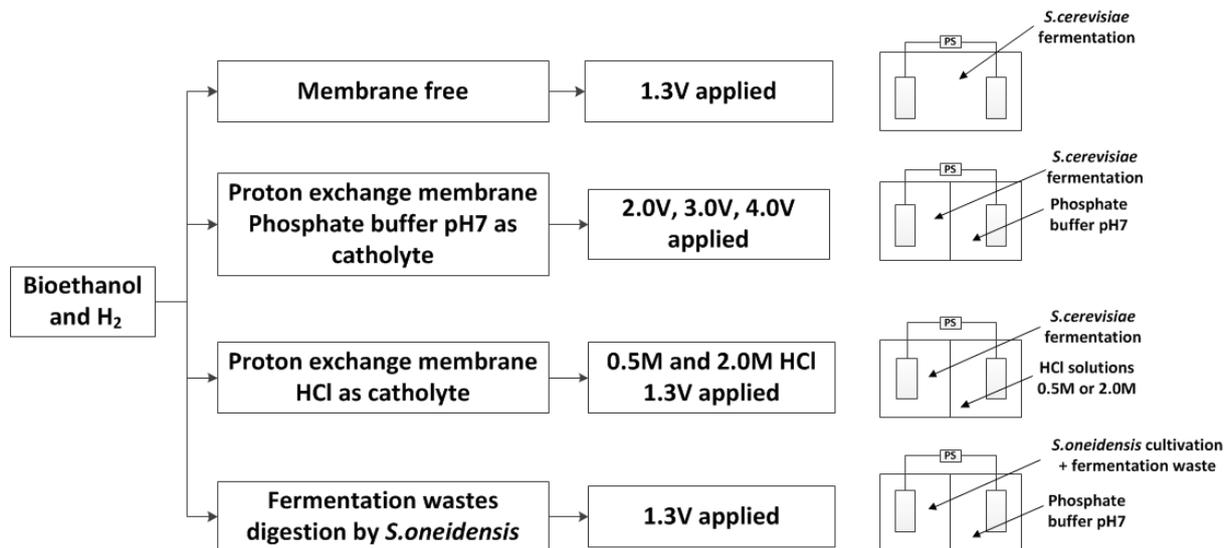
Figure 39: Diagram of experiments realised for hydrogen and bioethanol co-production.
