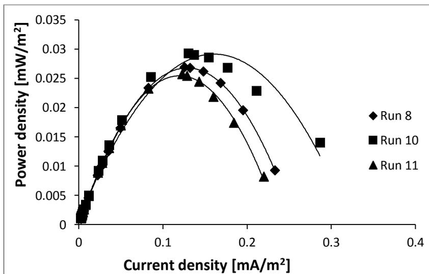
Figure 41: Power density curves normalized to the true surface area of the anode.
