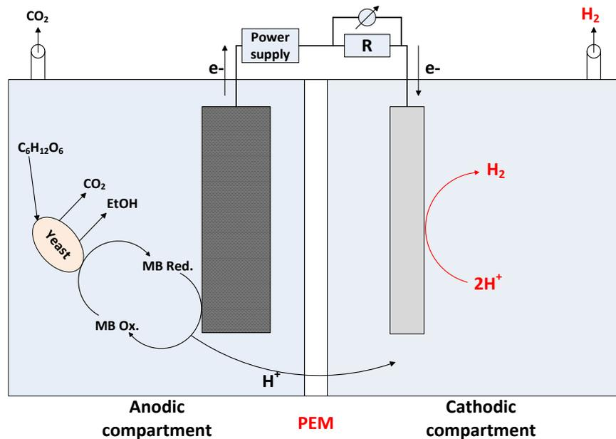
Figure 3: Microbial electrolysis cell principle. MB: Methylene Blue, mediator in the anode compartment. PEM: proton exchange membrane. R: external resistance. The final electron acceptors in the cathodic compartment are protons released in the anodic compartment.
