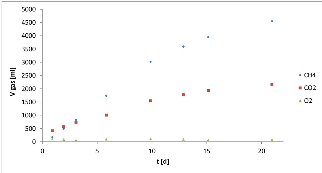
Figure 61: Gas production over the acclimation phase preceding the digestion of fermentation waste under 0V.
