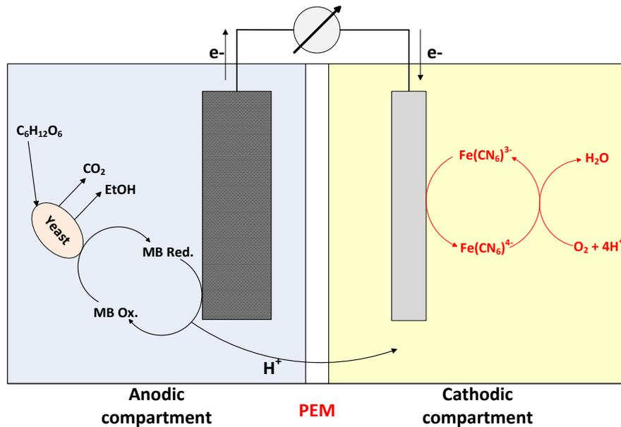
Figure 2: Microbial fuel cell principle. MB: Methylene Blue, mediator in the anode compartment. PEM: proton exchange membrane. The final electron acceptor in the cathodic compartment was potassium ferricyanide.
