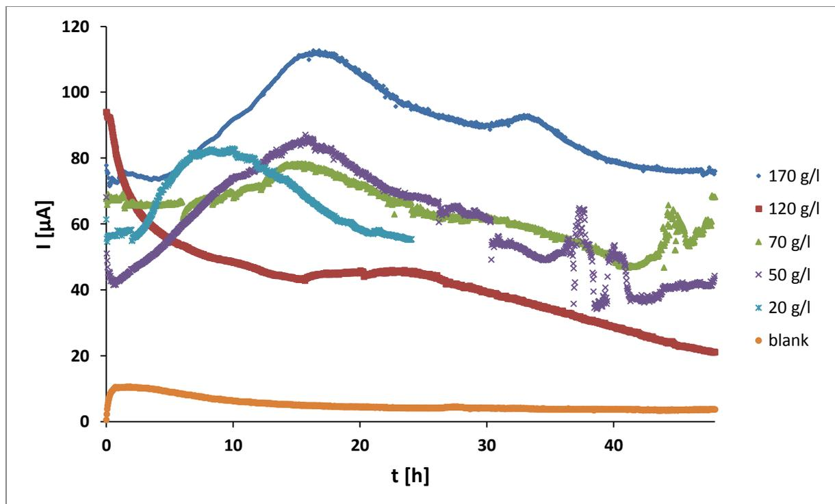
Figure 18: Currents recorded over time at different glucose concentration when the bioelectrical fuel cell was operated as microbial fuel cell without mediator. Blank = media oxidation without *S. cerevisiae*.
