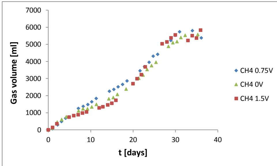
Figure 36: Methane production during the digestion of fermentation wastes under different applied voltage.
