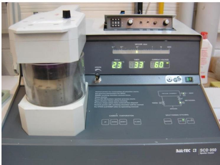
Photo 1: The Sputter coater device used for platinum deposition on reticulated vitreous carbon electrodes.
