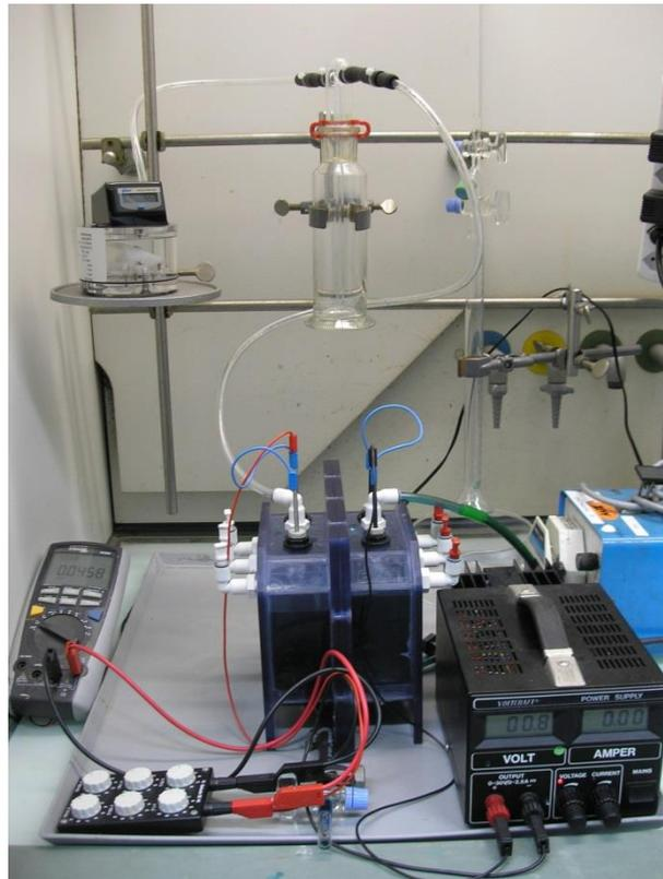
Photo 4: Set-up of the bioelectric fuel cell used in microbial electrolysis cell mode. A voltage was applied to the fuel cell by the power supply on the right, the gas produced was monitored by a milligas-counter placed above the reactor and the current was monitored by a multimeter (on the left) connected over an external resistance.
