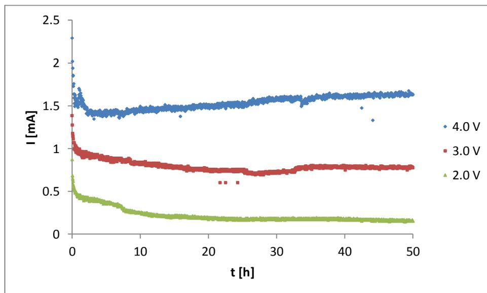
Figure 25: Currents recorded with 2.0, 3.0 and 4.0 V applied in the microbial electrolysis cell with a phosphate buffer as catholyte.
