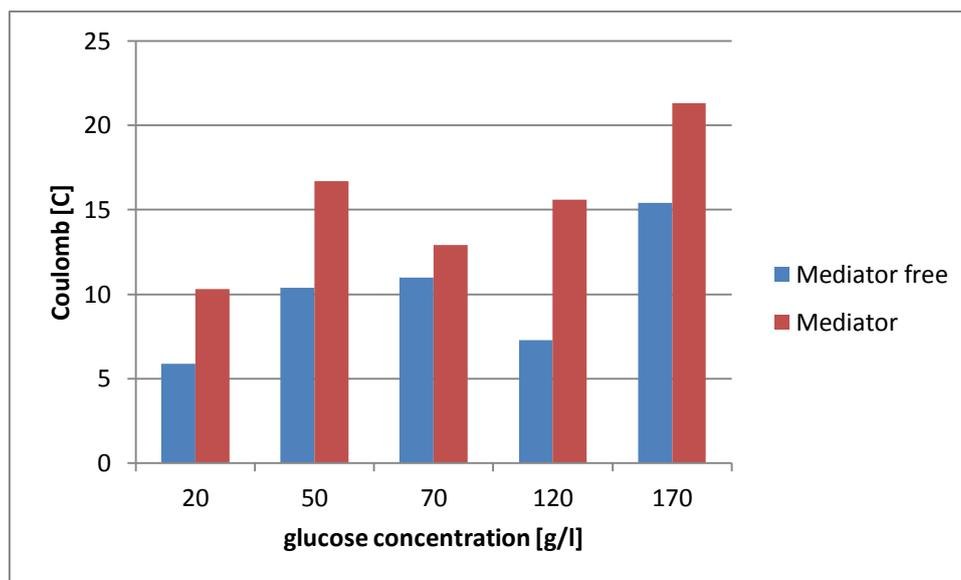
Figure 20: Number of coulomb generated with different initial glucose concentration in presence and absence of a mediator.
