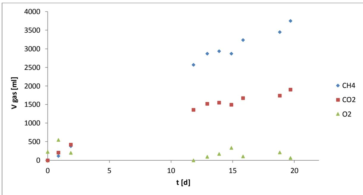
Figure 64: Gas production over the acclimation phase preceding the digestion of fermentation waste with in situ hydrogen production.
