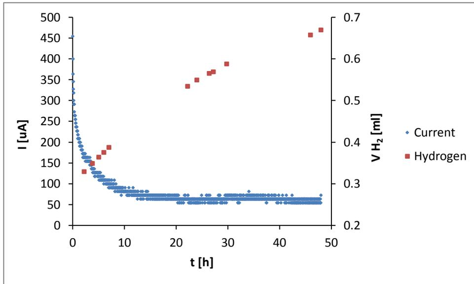
Figure 30: Current and hydrogen production in microbial electrolysis cell operated with a 2.0 M HCl solution as catholyte under 1.3 V of applied voltage, after overnight acclimatization of the fermentation.
