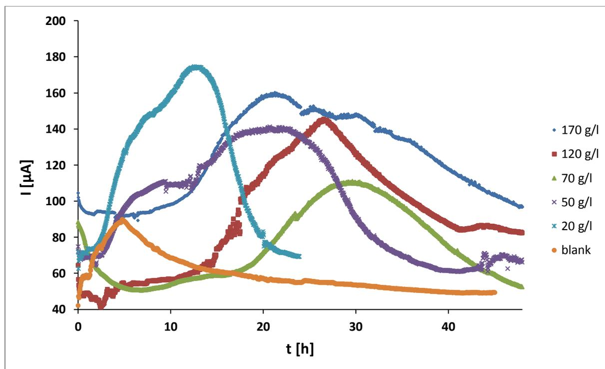
Figure 19: Currents recorded over time with different glucose concentration when the bioelectrical fuel cell was operated as microbial fuel cell with 0.3 mM of Methylene Blue as mediator. Blank = media oxidation without *S. cerevisiae*.
