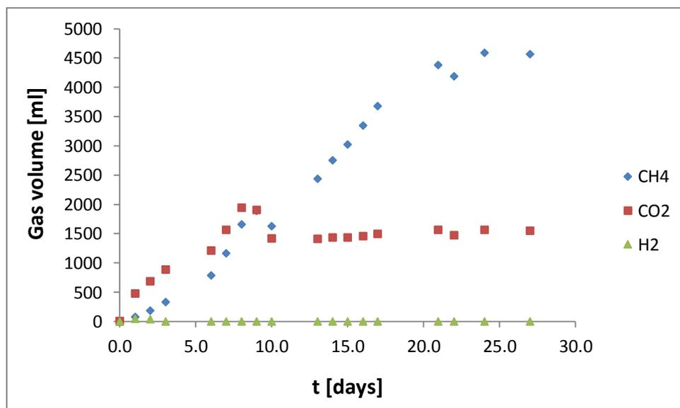
Figure 38 Gas composition in the headspace of the reactor over the in situ hydrogen production experiment.
