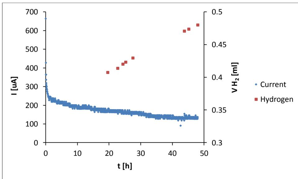
Figure 31: Current and hydrogen production in a microbial electrolysis cell operated with a 0.5 M HCl solution as catholyte and 1.3 V of applied voltage, after overnight acclimatization.
