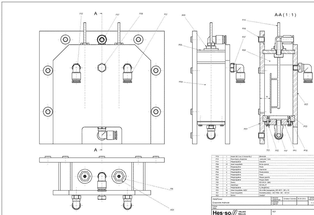
Figure 6: Plan of the cathodic compartment. The cathode including the external connections were made from pure nickel. The gas generated was collected through the quick connection on the top of the respective compartment. The quick connection on the bottom of the compartment was used to remove trace oxygen by sparging with nitrogen.
