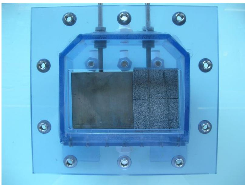
**Photo 3: Nickel cathode partially covered by platinized RVC electrodes (on the right). When the bioelectrical fuel cell was operated as a microbial electrolysis cell, the nickel cathode was completely covered with this type of electrodes.**
