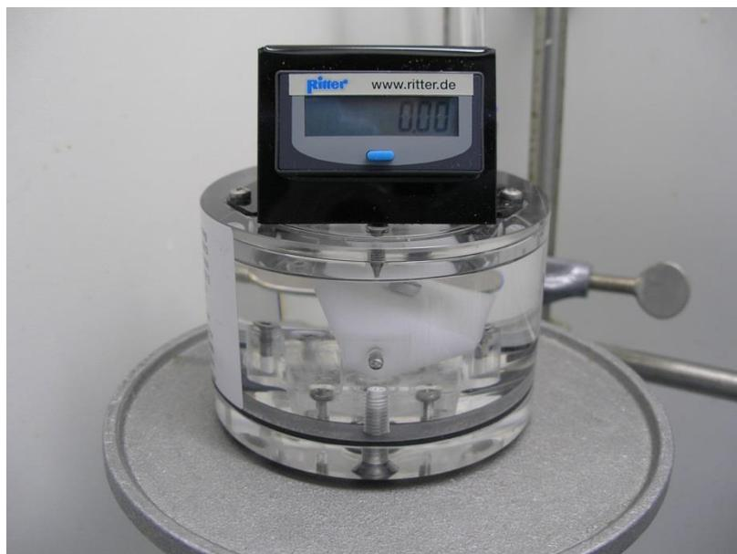
Photo 5: MGC-1 V3.2 PMMA Milligas-counter filled with silicone oil to monitor gas volumes produced in the cathode compartment.
