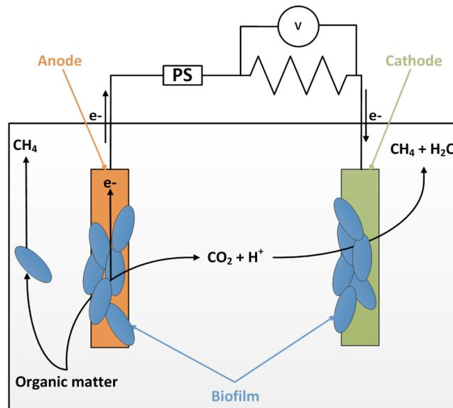
Figure 4: Methane production from fermentation wastes. Carbon dioxide is converted into methane through in-situ hydrogen production.
