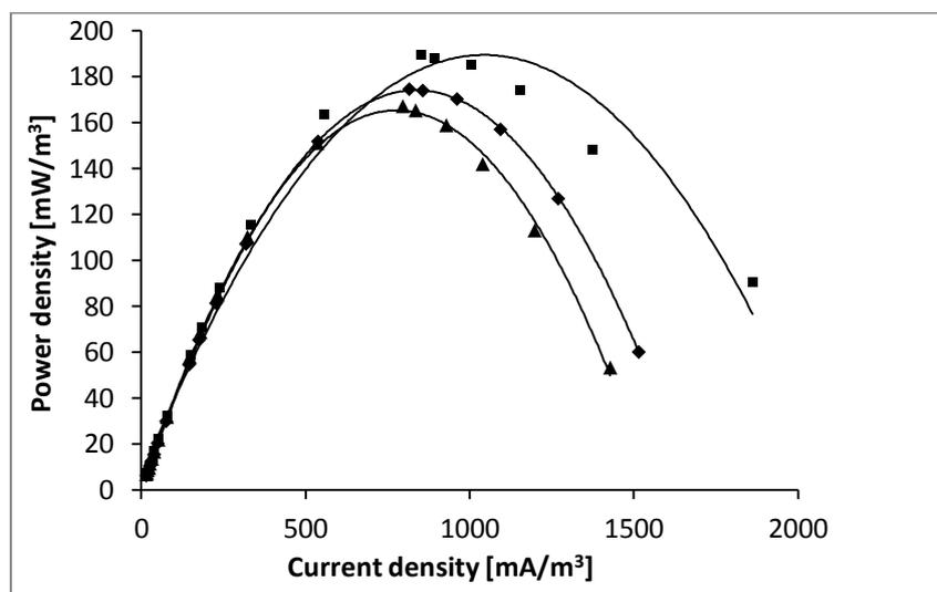
Figure 14: Power density curves normalized to the anode volume. The power densities were measured from three distinctive *S. cerevisiae* cultivations and renewed catholyte.
