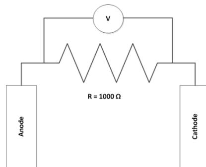
Figure 9: Electrical diagram for current production and monitoring in microbial fuel cell mode.
