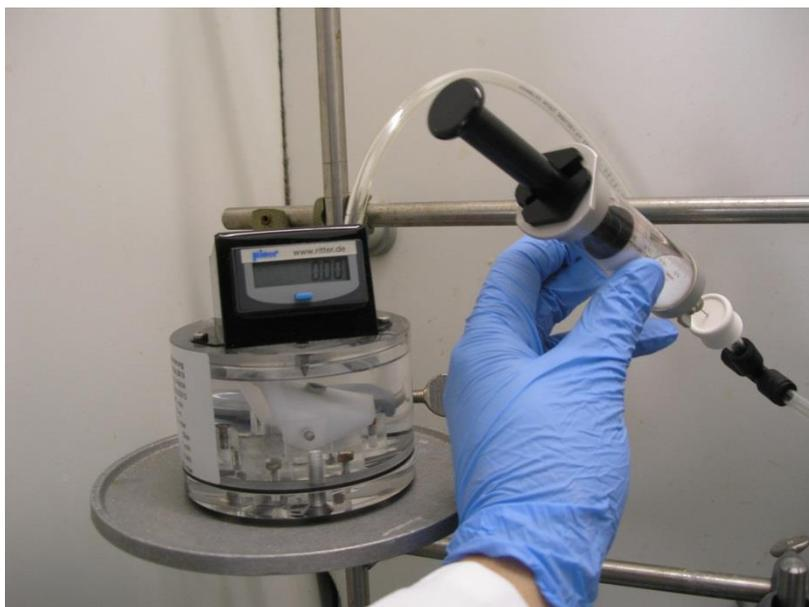
Photo 6: Withdraw of a gas sample through a folding skirt stopper on the gas tight tubing connecting the milligas-counter and the cathodic compartment. The gas samples were taken with a gas tight syringe.
