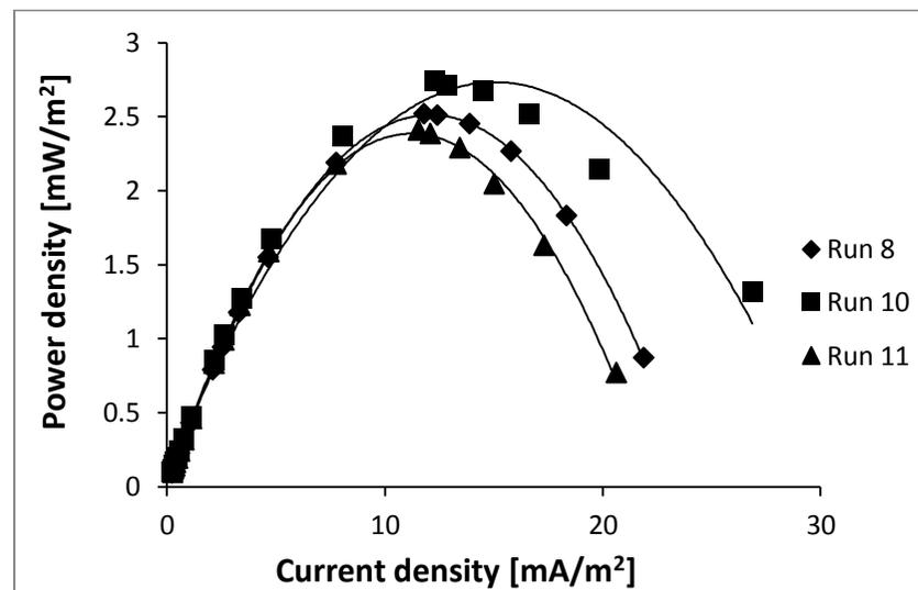
Figure 42: Power density curves normalized to the anode opposite surface area.
