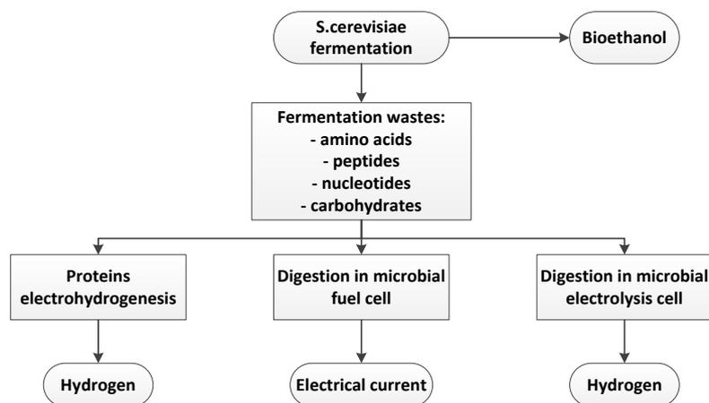
Figure 40: Valorisation of fermentation waste with bioelectric fuel cell system.
