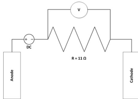
Figure 11: Electrical diagram for current and hydrogen production in microbial electrolysis cell mode.
