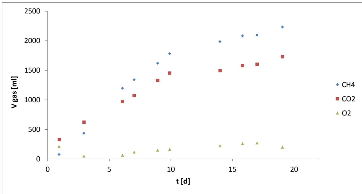
Figure 62: Gas production over the acclimation phase preceding the digestion of fermentation waste under 0.75V.
