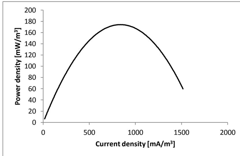
Figure 8: Example of a power density curve, the top of the curve corresponds to the maximum power output.
