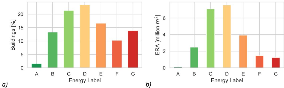
Figure 8: a) Energy label distribution by share of buildings and b) by energy reference area (both according to the CECB dataset).
