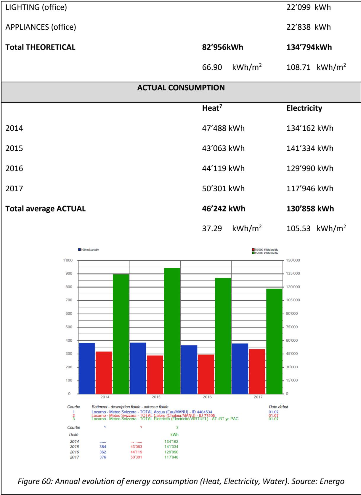
Figure 60: Annual evolution of energy consumption (Heat, Electricity, Water). Source: Energo
