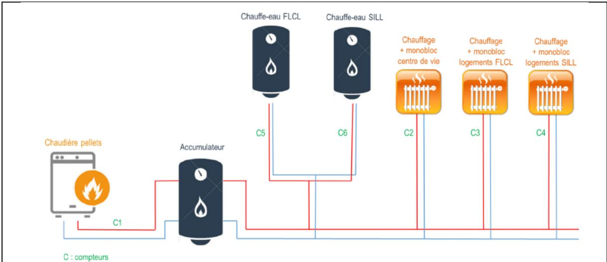
Figure 50: Position of heating meters. Source: Ergo
