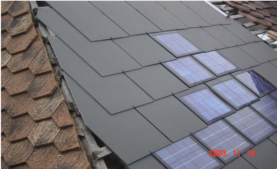
Figure 6 shows the test stand at the premises of the roofer Georg Achermann in Schwyz. The test set up was to evaluate changes and the interwiring concept. The shingles were modified to the chosen size of 40cm by 72cm. The test stand allowed easy checking of the cabling at the back side of the modules (Source G. Achermann, roofer, Schwyz)
