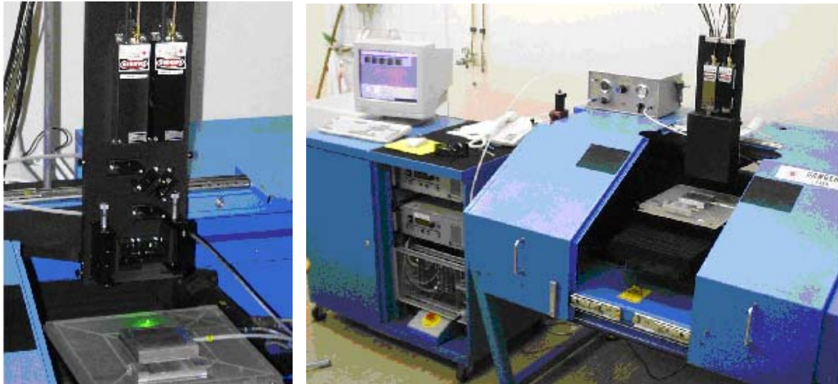
Fig. 29: IMT's updated "old" laser scribing system (originally donated by Industry), containing now the two new diode lasers ( \lambda = 1064 \text{ nm} & 564 \text{ nm} ).
