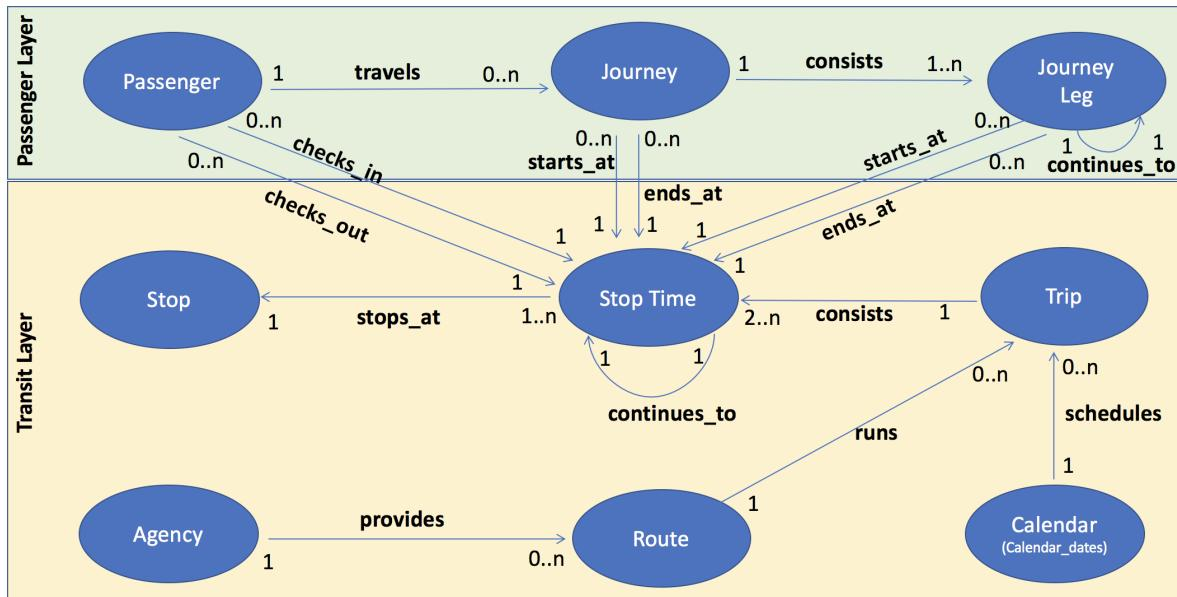
This is a Graph-based data model, which is the underlying structure of a Graph Database as explained below in Section 2.4. The numbers at the heads and tails of the edges (blue arrows) indicate whether the edge represents a one-to-one, a one-to-many, many-to-one or a many-to-many relationship, similar as in standard entity-relationship-diagrams. For example, a trip consists of many (but at least 2) stop time objects, while a stop time object can be associated to exactly one trip.
