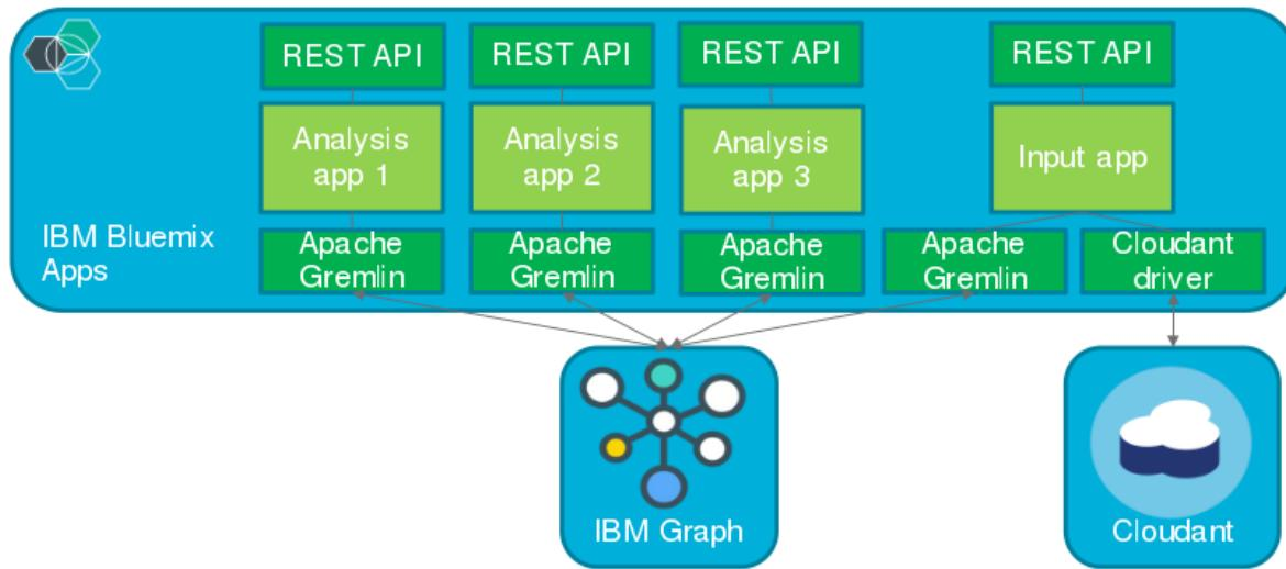
The application is designed as a web application running on IBM Bluemix, a Platform-as-a-Service (PaaS) built on Cloud Foundry, an open source, multi cloud application platform as a service. The data backend of the application is IBM Graph, a Database-as-a-Service (DBaaS) running on IBM Bluemix. IBM Graph is a graph database with support for Gremlin and implements the data model described above.
