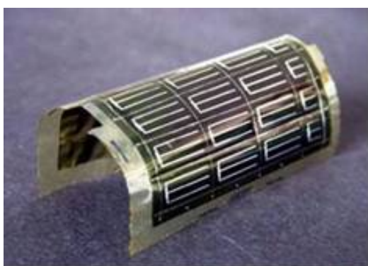
Figure 1: Flexible CIGS solar cells on a 5 x 5 cm 2 polyimide foil (left) and current-voltage characteristic of the 14.1% efficiency cell measured under simulated AM1.5 standard test conditions at ISE-Fhg Freiburg, Germany (right). This value still remains the highest efficiency record for any kind of solar cell grown on polymer foil.
