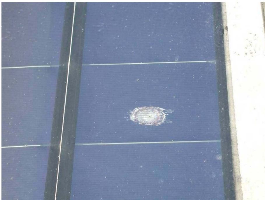
Figure 28: Fissure on module front surface with water infiltration (1st module at north side of string 1).
