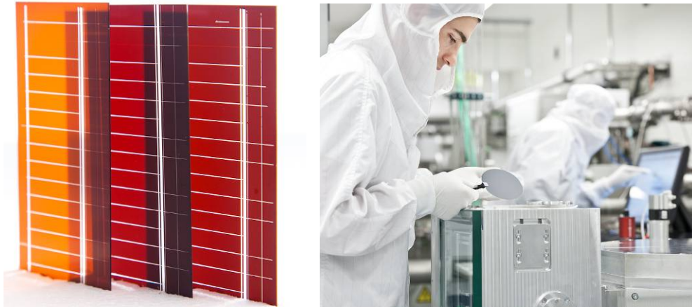
Figure 17: Amorphous mini-modules obtained by laser patterning and monolithic integration (left). Test coating on a the new Indeotec cluster system (right)
