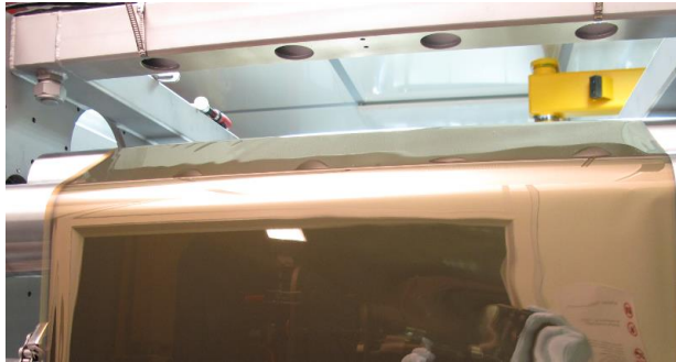
Figure 7: rewinding zone with copper coated web after a copper deposition test.
