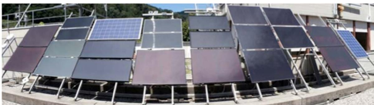
**Figure 5.1:** Picture of the outdoor testing facility at ISAAC with the 11 different thin film technologies and 2 c-Si modules for inter-comparison.
