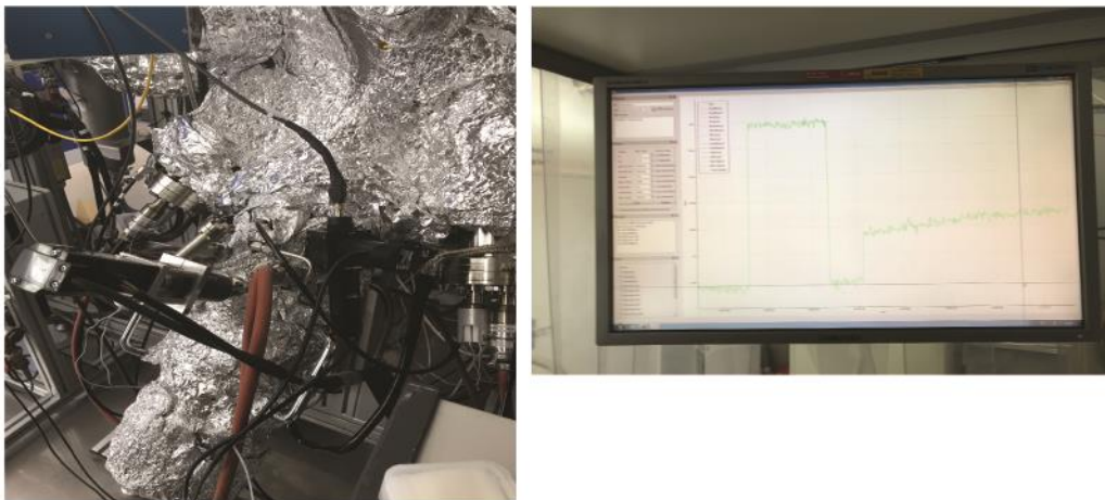
Figure 1: Photograph of the Flux-Monitor installed on the evaporation chamber and the GUI shown on the right.
