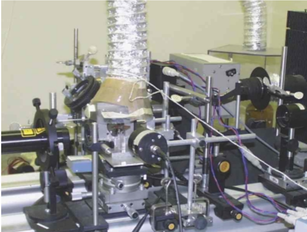
Fig. 29: PDS and CPM setup sharing the same light source (halogen lamp and monochromator).
