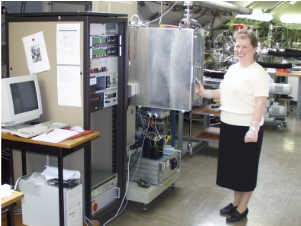
Fig. 26: Computer controlled automatic 30cm x 30cm VHF-plasma deposition reactor for fabrication of amorphous silicon solar cells.
