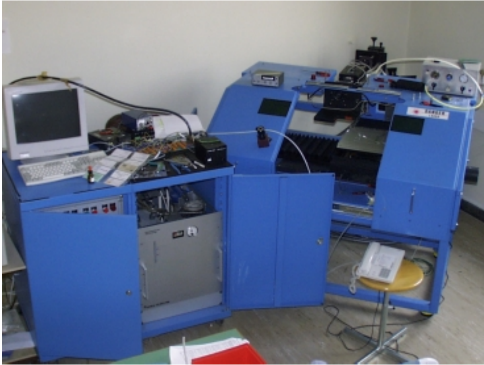
Fig. 27: Laser scribing system for structuring and series connection of thin film solar cells, including pulsed YAG laser and computer controlled 30cm x 30cm xy-table. This equipment has been donated to IMT by an industrial partner. It was upgraded in-house to comply with the special needs of IMT's device technology.
