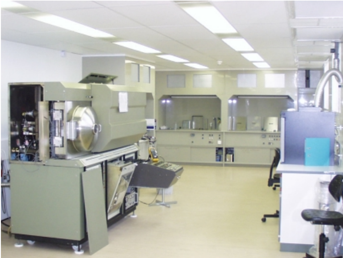
Fig. 24: Class 10000 cleanroom of 60\text{ m}^2 area on the second floor of the Breguet 2 building. In the wet-bench areas with laminar flow, class 100 conditions can be obtained for critical operations.
