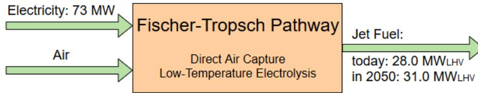
**Figure 6.** Block flow diagram with preliminary mass and energy balance for the conversion of carbon dioxide from air to jet fuel, via the Fischer-Tropsch pathway with direct air capture and low-temperature electrolysis. Output values: today and forecast for 2050 (Schmidt et al., 2018).
