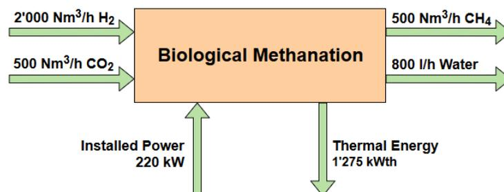
**Figure 3.** Specification of a biological methanation based on Electrochaea's BioCat methanation plant. Reactor temperature is 63 °C, reactor pressure is 10 barg.
