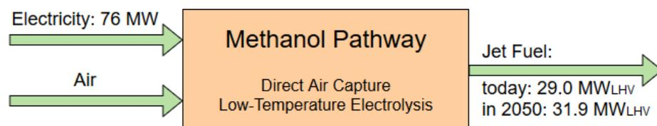
**Figure 5.** Block flow diagram with preliminary mass and energy balance for the conversion of carbon dioxide from air to jet fuel, via the methanol pathway with direct air capture and low-temperature electrolysis. Output values: today and forecast for 2050 (Schmidt, et al., 2018).
