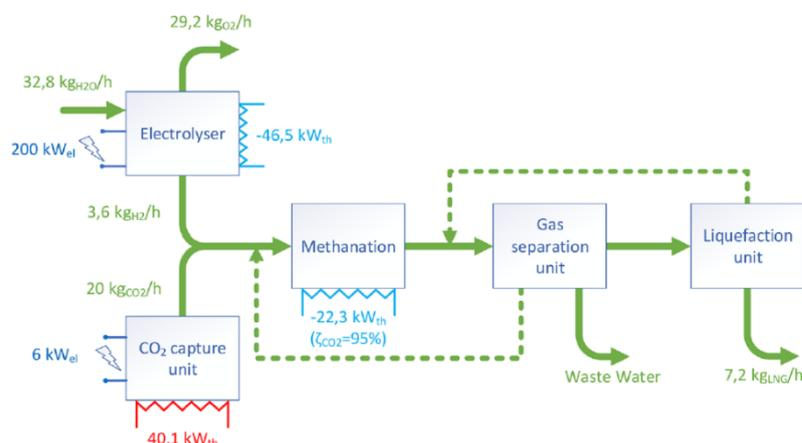
**Figure 2.** Block flow diagram with preliminary mass and energy balance for the conversion of carbon dioxide (from air) and hydrogen to LNG (Morosanu, et al., 2018).
