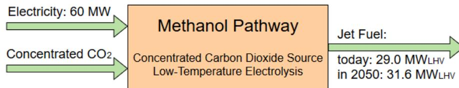
**Figure 7.** Block flow diagram with preliminary mass and energy balance for the conversion of carbon dioxide from a concentrated CO<sub>2</sub> source to jet fuel, via the Methanol pathway with low-temperature electrolysis. Output values: today and forecast for 2050 (Schmidt et al., 2018)
