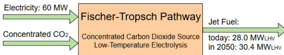
**Figure 8.** Block flow diagram with preliminary mass and energy balance for the conversion of carbon dioxide from a concentrated CO<sub>2</sub> source to jet fuel, via the Fischer-Tropsch pathway with low-temperature electrolysis. Output values: today and forecast for 2050. (Schmidt et al., 2018)
