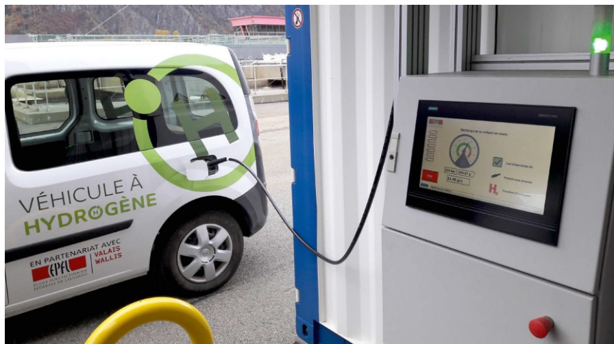
Figure 21 - User friendly interface for the automated 350 bar refueling sequence
