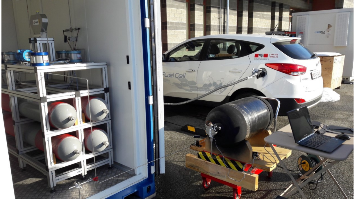
Figure 22 - High pressure tank testing with hydrogen recycling
