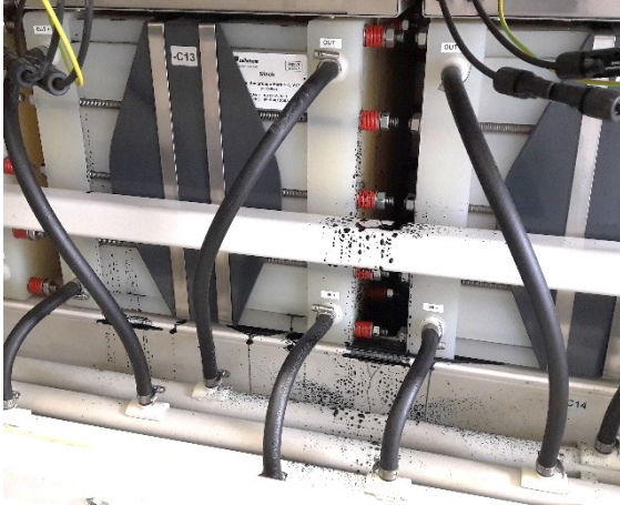
Figure 3 - Leakage of electrolyte in the system and stack disassembly in the lab
