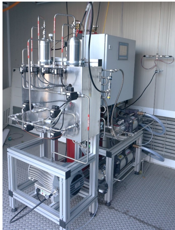
Figure 12 - Purification and compression system
