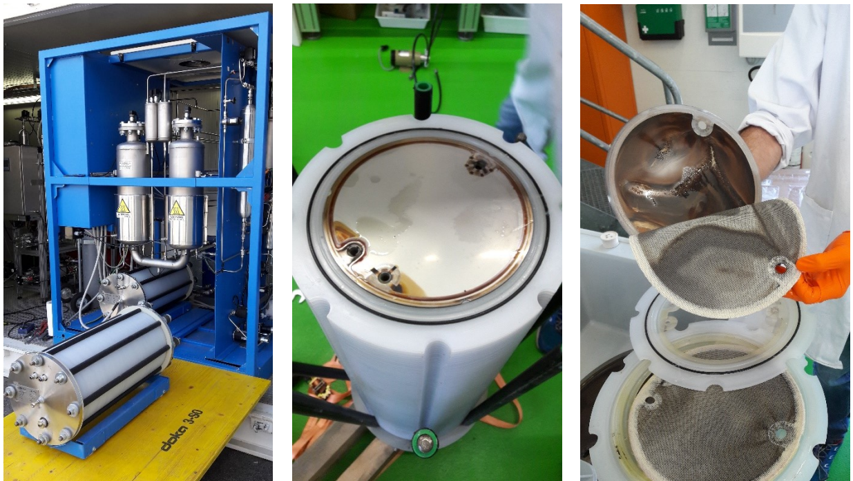
Figure 10 - Alkaline stack replacement and disassembly
