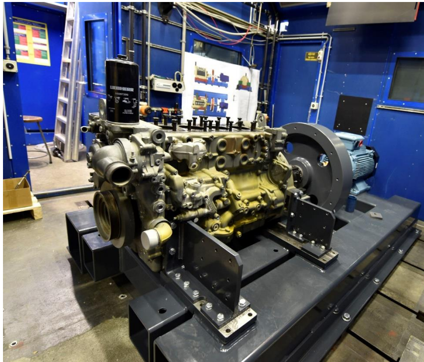
Figure 44: An image from the lab during assembly of the test rig drive train. The combustion chamber / cylinder head is not yet mounted on the engine block.
