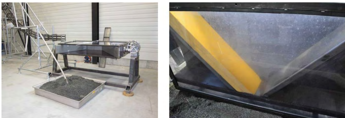
Fig. 2.10: Left hand: Test box in horizontal position with already installed panel sheets. Right hand: Test box in upside down position ready for filling with soil material. Insulating wall panels (in yellow) had been used for varying the crest's dimension without changing the slope inclination.
