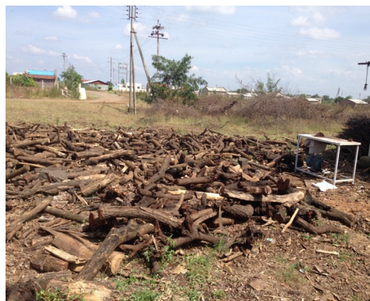
Figure 2: wood collected at plant site for sizing and use in gasifier
