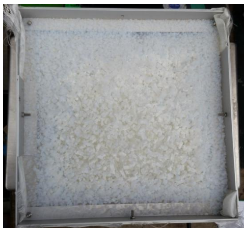
Figure 15: Granulate after drying for 40 minutes at 150°C.
