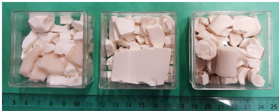
Figure 3. Silica-pectin hybrid aerogels prepared by APD from heptane-HMDSO at 65/150°C.
