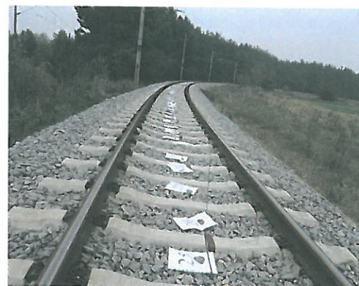
fig. 7 Instrumented hammer, accelerometers + marked inner-sleeper space
