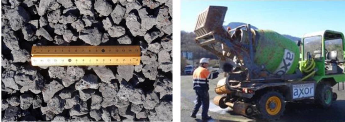
While this method will allow for large scale production, only a limited sphericity of the EAF slag pebbles within the acceptable tolerance can be established with an overall efficiency of around 60% and a discarding rate of 40%. Nevertheless, the mechanical conformed method represents a feasible alternative to produce slag pebbles in a cost effective way and the produced pebbles will be tested in the pilot plant.
