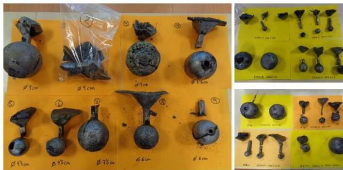
Additionally, the production of large amounts of pebbles presented significant limitations due to the high viscosity of the slag melt, ultimately leading to the conclusion that this method is not technically or economically feasible.
