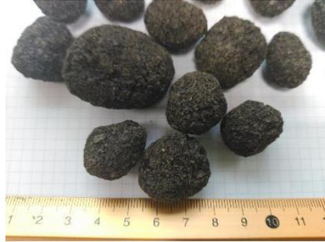
Using this method, a large amount of slag pebbles can be produced with favorable characteristics and the sintered slag pebbles will be tested in the Slagstock pilot plant (WP4).
